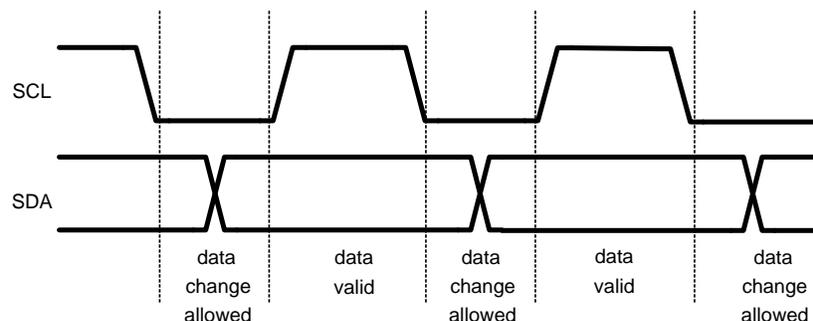
**Figure 3. I<sup>2</sup>C Signals: Data Validity**
