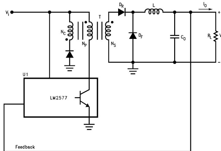
**Figure 1. Basic Forward Converter**
