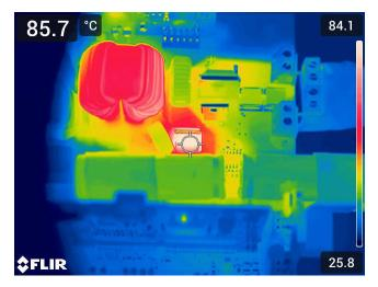
Figure 4-31. Relay Bypass Switch Thermal Image
