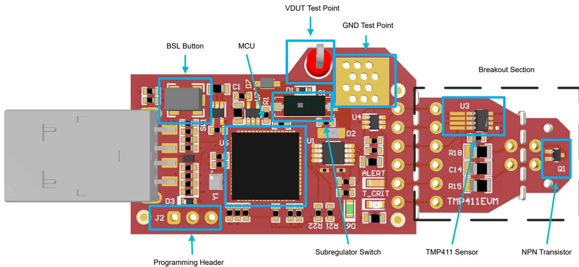
Figure 2-1. TMP411EVM Board Sections
