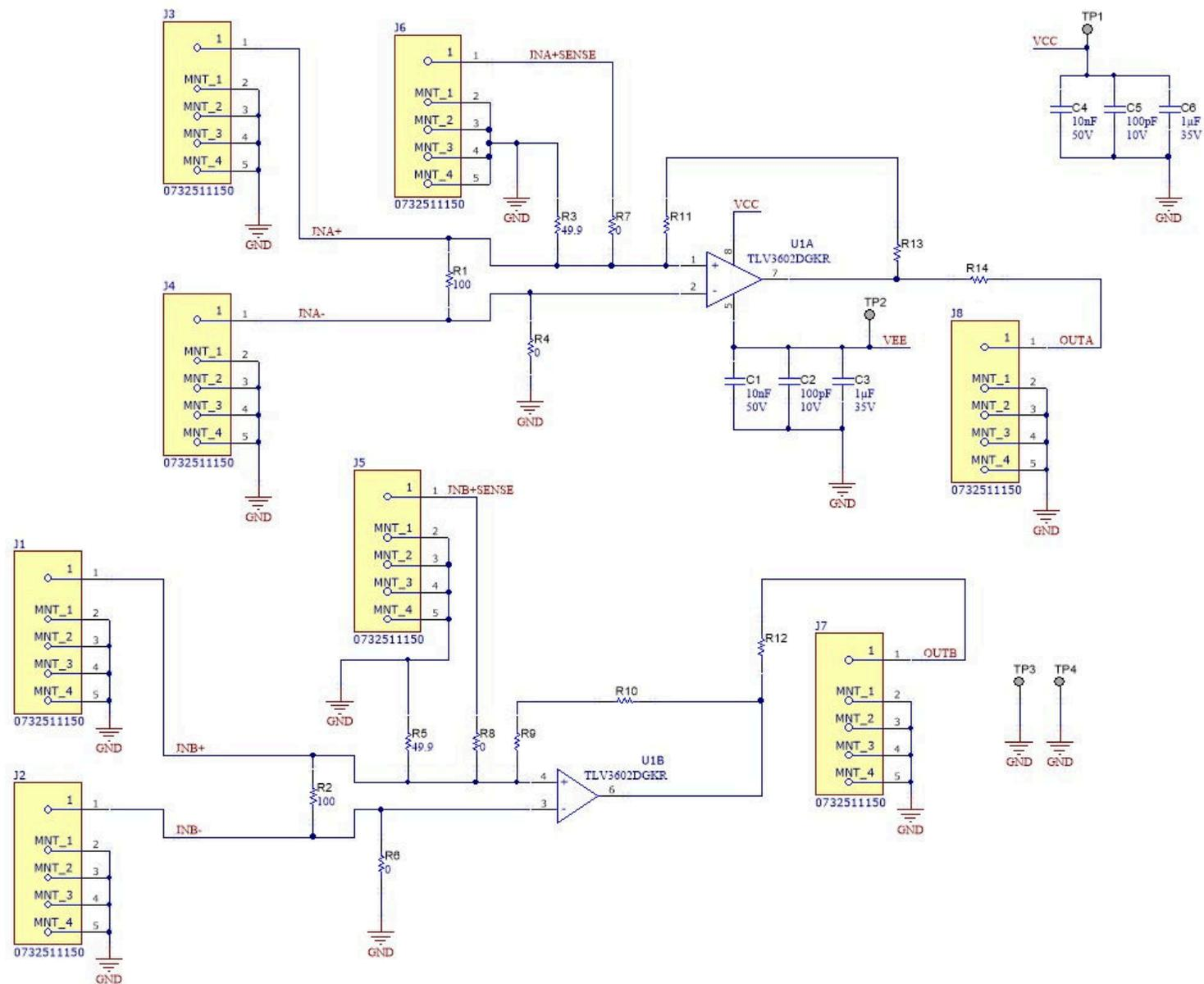
Figure 7-1. TLV3602EVM Schematic
