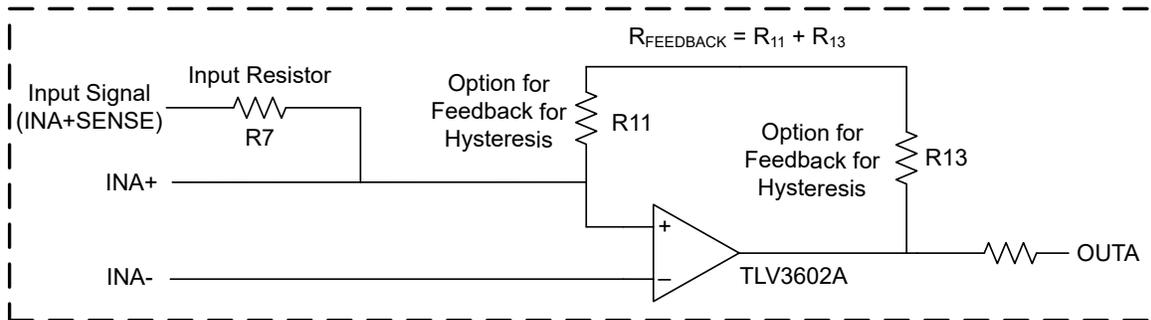
**Figure 5-5. TLV3602 Hysteresis Schematic for Channel A**
