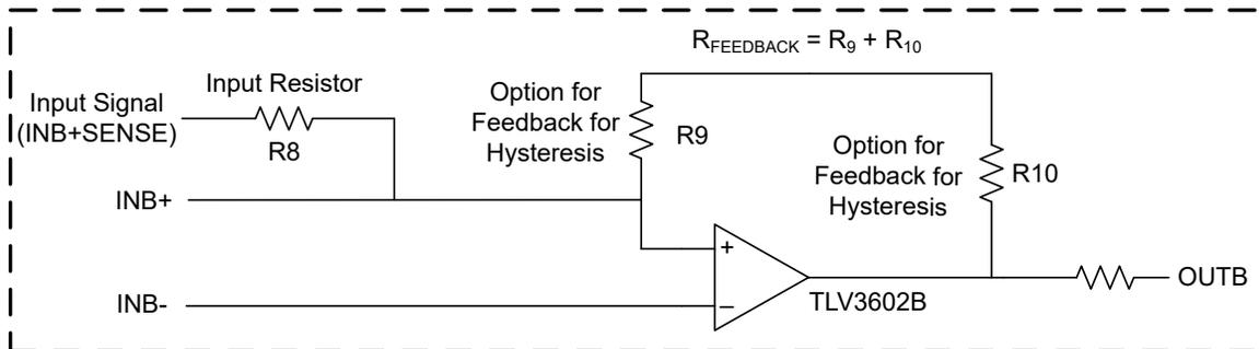
**Figure 5-6. TLV3602 Hysteresis Schematic for Channel B**
