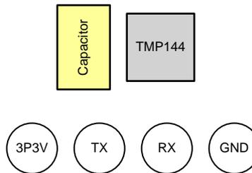
Figure 2. TMP144EVM Pin Connections
