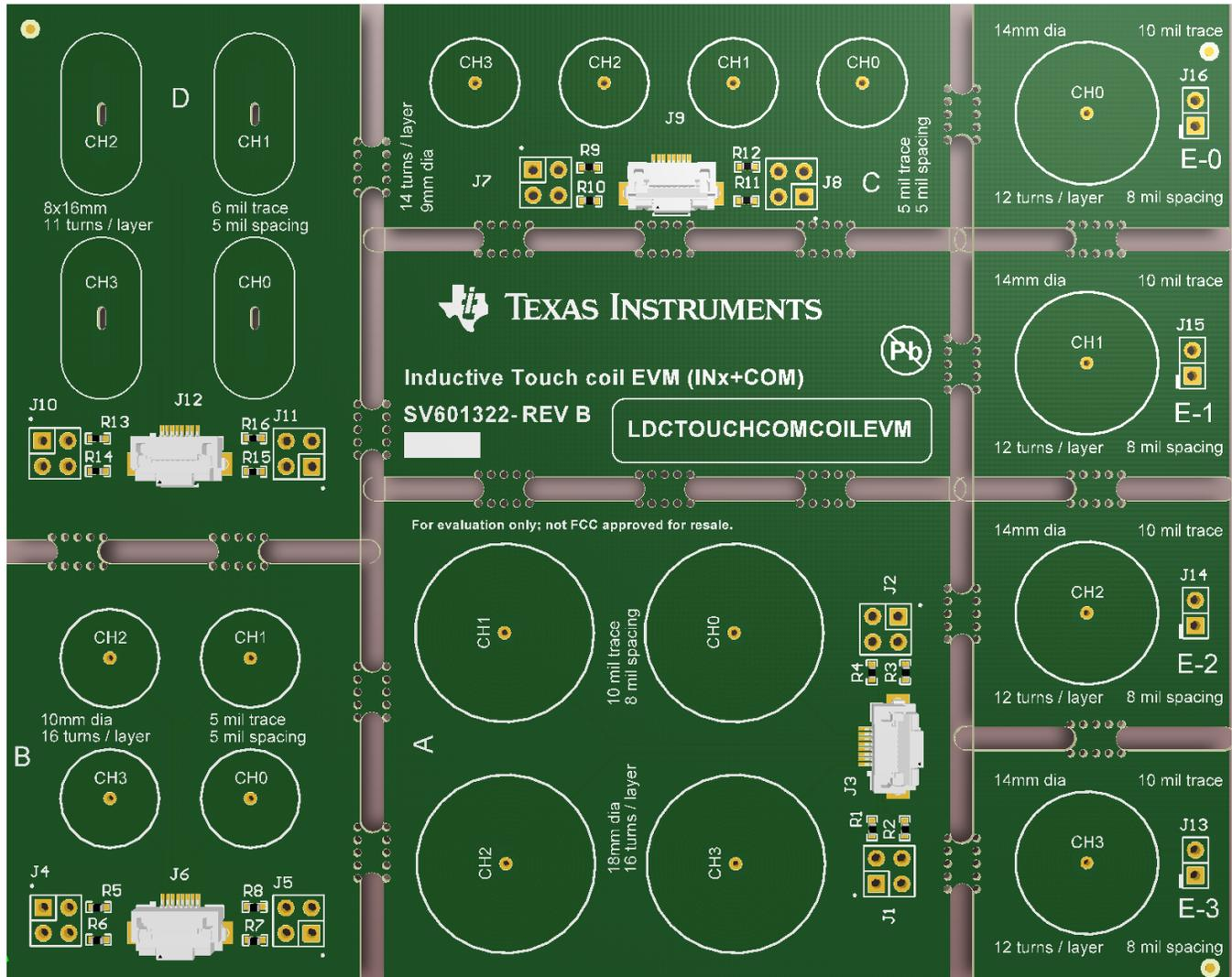
Figure 1. LDC Reference Coils Board (Top View)
