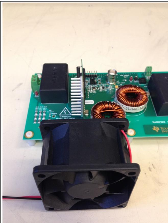
Figure 10. Recommended Configuration for Heatsink and Fan
