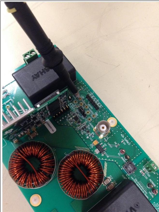
Figure 8. Recommended Probe Connection for Logic Signals
