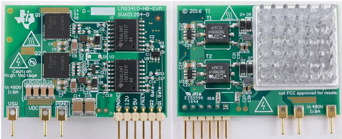
Figure 2. Front and Back Side Photos of LMG3410-HB-EVM
