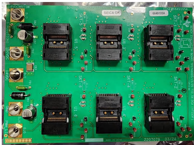
Figure 2-1. HDR TID Hardware
