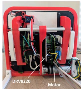
**Figure 3-2. Rear View of Door Handle Demo**
