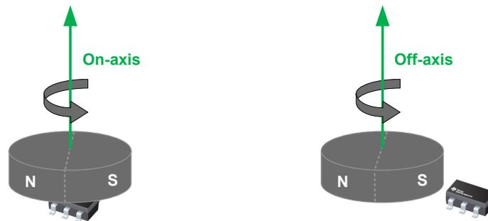
Figure 4-8. On-Axis vs. Off-Axis Sensor Alignment
