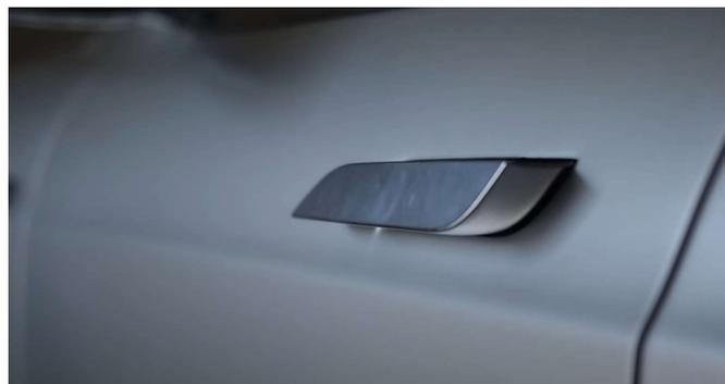
**Figure 2-1. Deployable Door Handle in Extended Position**
