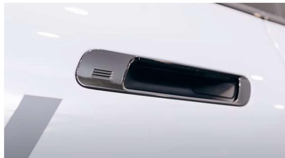
**Figure 2-3. Recessed Cavity for Fixed-Flush Door Handle**
