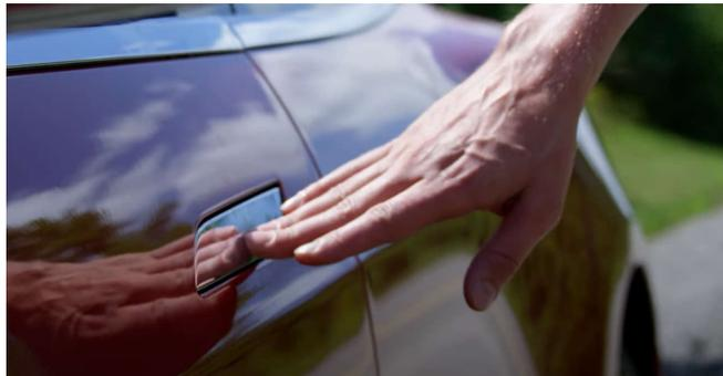
**Figure 2-2. Soft-Touch or Hand Proximity Detection for Deployable Door Handle**
