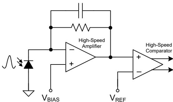
Figure 2. Pulse Receiver Circuit
