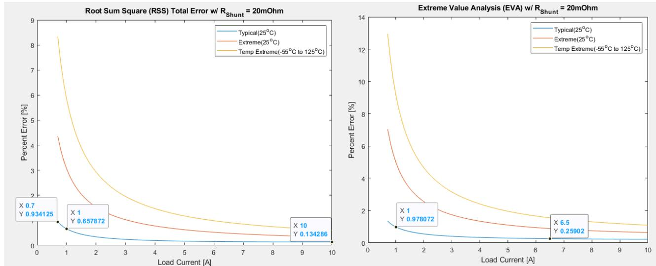
The RSS is 0.658% when the load current is 1 A. This RSS satisfies the 0.7% error requirement. The EVA plot is also provided on the right as a reference.
