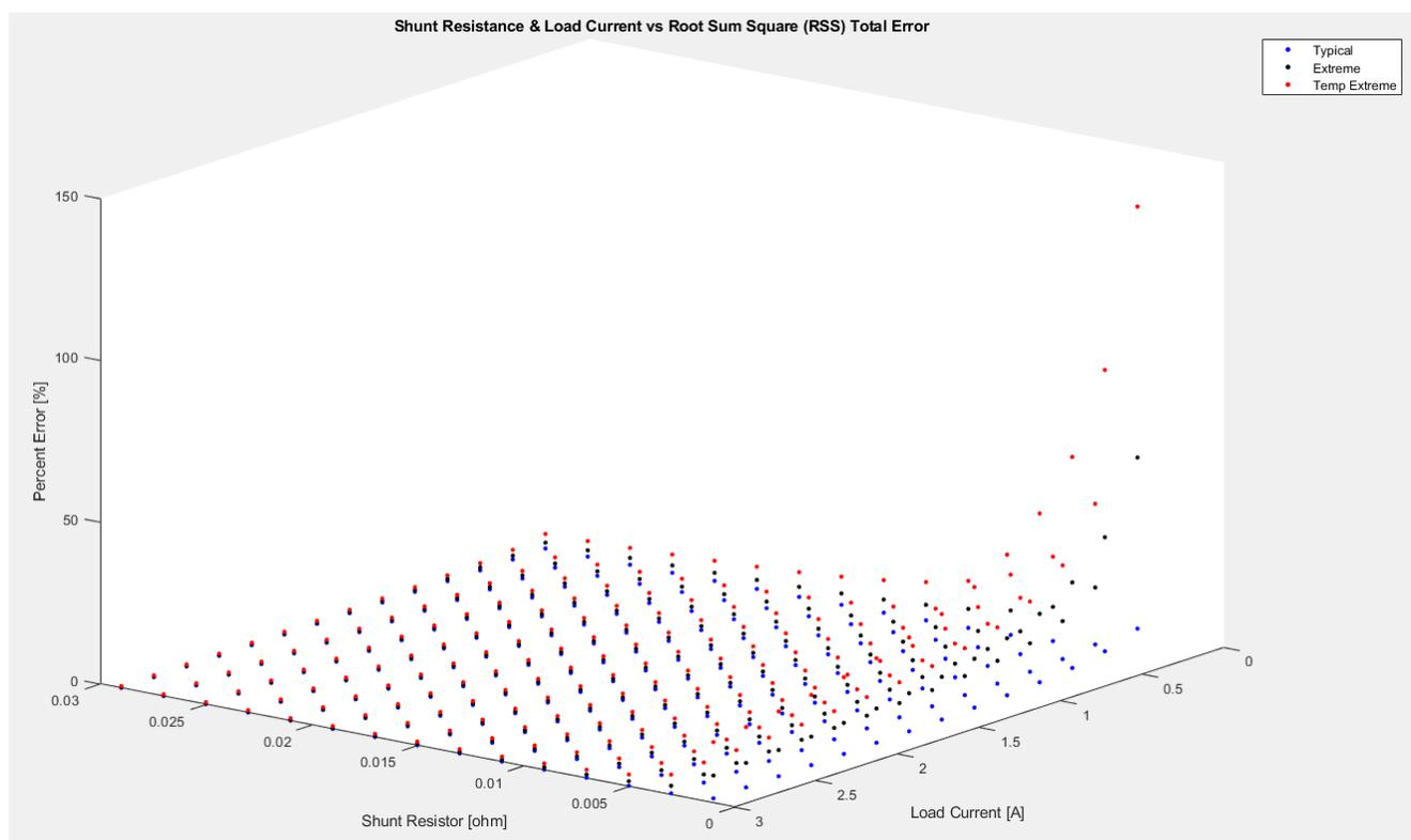
As shown in the previous image, the shunt resistor ( $R_{shunt}$ ) and load current ( $I_{load}$ ) are used as the inputs for calculating the output percent error. The result shows that the output percent error increases as  $I_{load}$  decreases or  $R_{shunt}$  decreases. Hence, the load current is set to its minimum value (1 A) when picking the  $R_{shunt}$  value to satisfy the minimum requirement in the specification.
