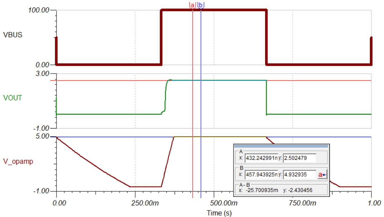
$V_{opamp}$ , which is the difference between  $V_{bus}$  and  $V_{EE}$ , is always below 4.933 V. LMP7704 is designed for a power supply up to 12 V, so it will not be damaged. Load current is set to 5 A in the simulation. As expected,  $V_{out}$  is simulated to be around 2.5 V.
