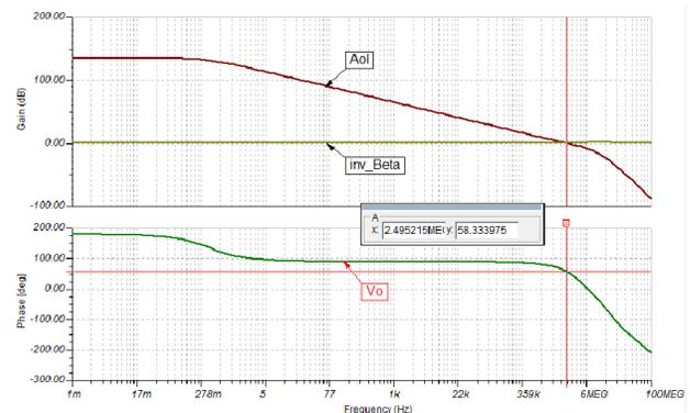
The previous image shows the frequency domain simulation result. The phase margin is measured at a point where  $1/\beta$  and Aol intersect, and it is 58.3 degrees, indicating the system is stable.
