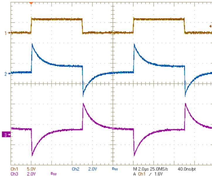
The following scope plot shows the propagation delay from the input of the driver to the output of the receiver. It is about 60 ns.
