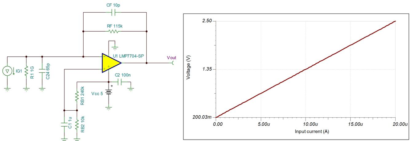
For zero input current, the simulated output voltage is 200.032 mV, and at 20- $\mu\text{A}$  input current, the simulated output voltage is 2.500 V and the gain is 115 kV/A.
