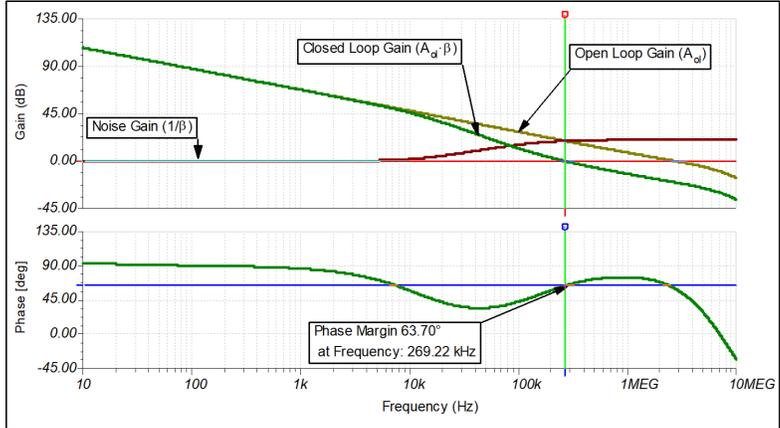
The loop gain plot shows the loop closure point (loop gain is 0 dB) at 269.22 kHz with 63.70 degrees of phase margin.
