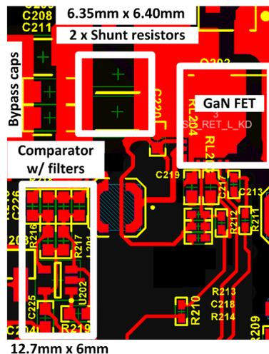
**Figure 3. Example Board Layout of a Discrete Shunt Resistor Implementation**
