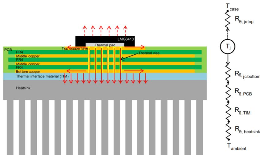
**Figure 1-1. QFN Package on a PCB (Green), TIM (Blue) and Heat Sink (Gray)**
