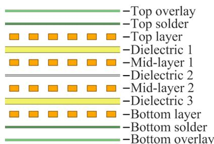
**Figure 2-2. An Example Layer Stack of a 4-Layer Board**
