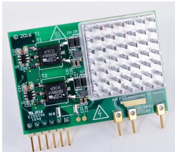
**Figure 3-1. 1.2-kW Half-Bridge Design**
