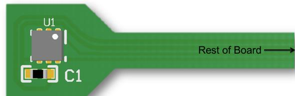
**Figure 1. TMP117 (U1) on Flex PCB, using an extended arm isolates the IC from being influenced by heat from other devices.**
