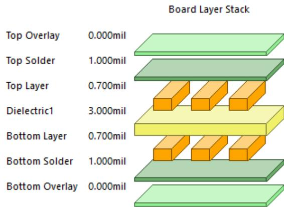
**Figure 2. Example flex layer Stack, thickness should be minimized to reduce thermal mass.**
