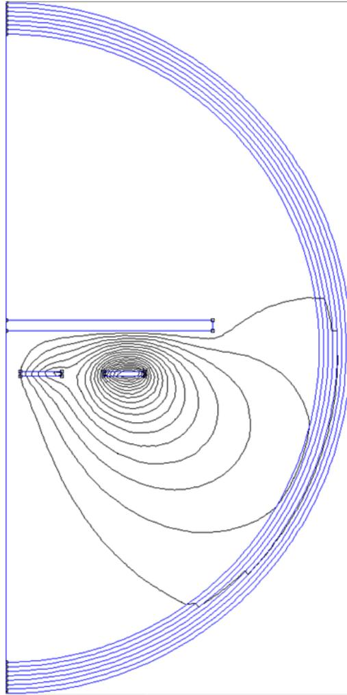
**Figure 3-1. Axisymmetric Answer File Showing the Contour Plot of the Magnetic Field Around the Coil and the Target**
