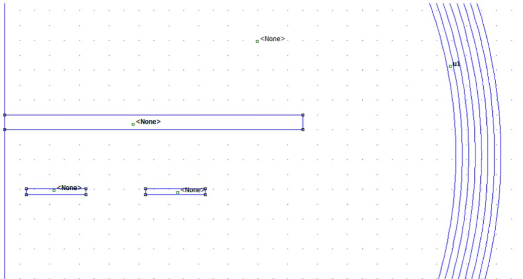
**Figure 2-8. Axisymmetric Problem Workspace With Block Labels**
