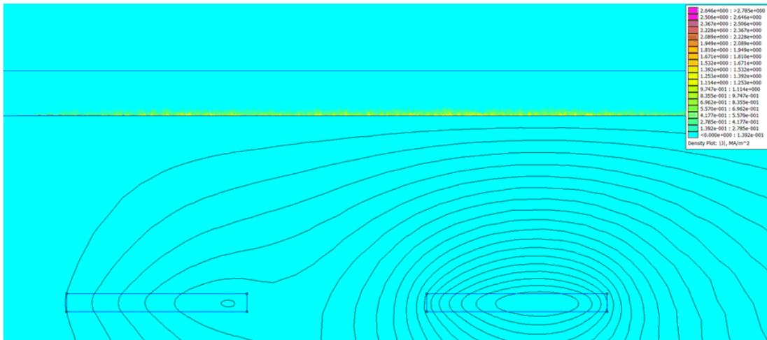
**Figure 3-4. Axisymmetric Answer File Showing Current Density Plot That Shows Eddy Currents on the Target**
