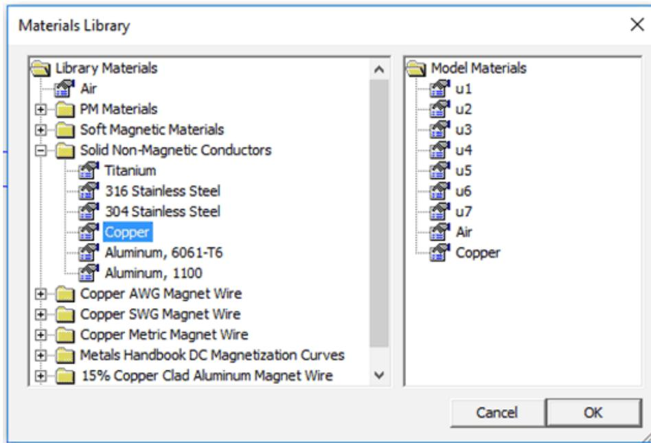
**Figure 2-10. Materials Library With Air and Copper Added to Model Materials**
