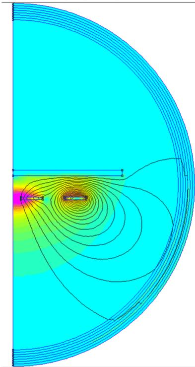
**Figure 3-3. Axisymmetric Answer File Showing Flux Density Plot**
