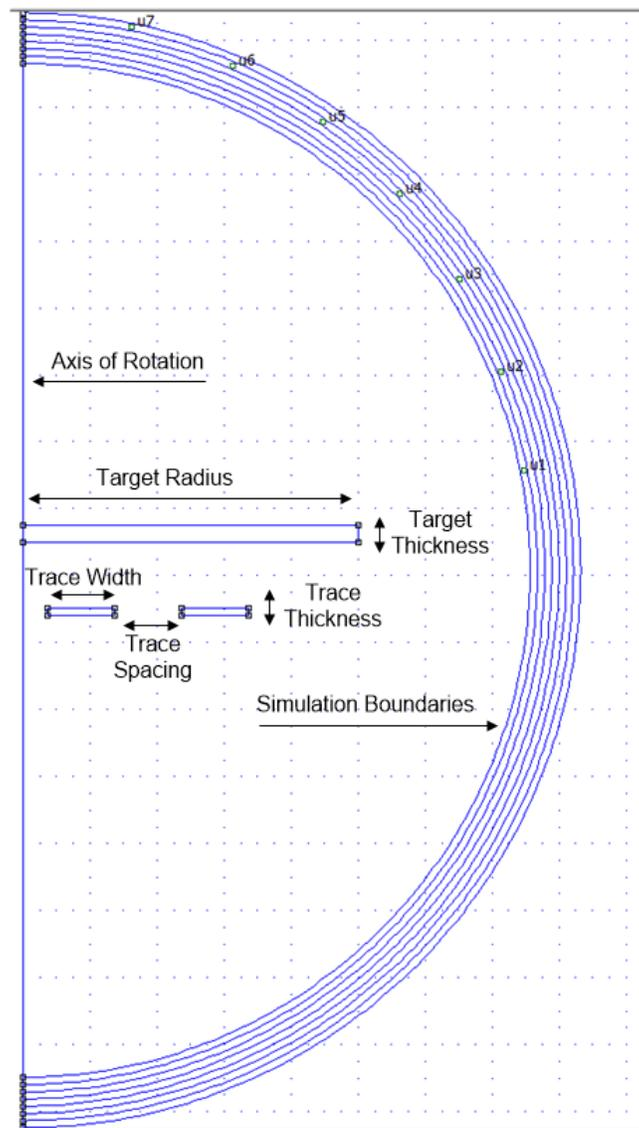
**Figure 2-3. Example Axisymmetric Problem Workspace With Labeled Traces and Target**
