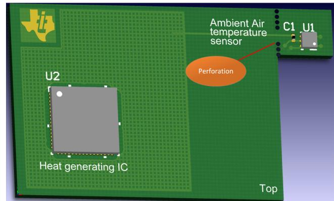
Figure 6. Perforated PCB Layout
