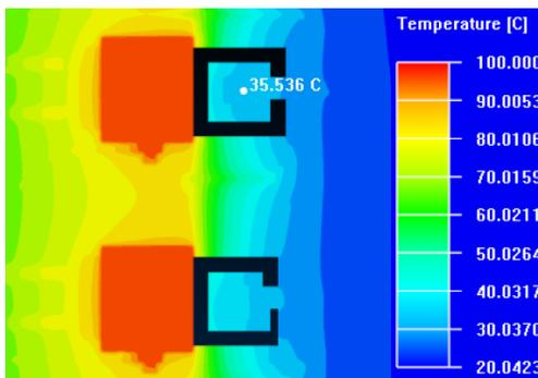
Figure 4. Thermal Air Gap With 1.8-mm Slot Width
