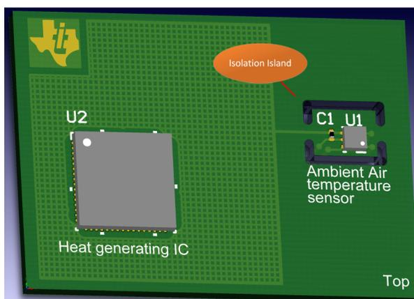
Figure 5. Isolation Island PCB Layout
