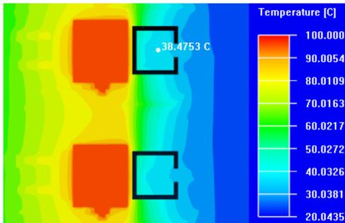
Figure 3. Thermal Air Gap With 0.8-mm Slot Width
