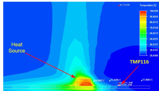
Figure 2. Heat Radiated Across Test Board
