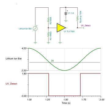
Figure 5. Precision Voltage Monitoring Simulation
