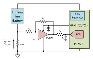
**Figure 2. Precision Current Monitoring**
