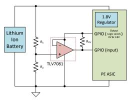
Figure 4. Precision Voltage Monitoring
