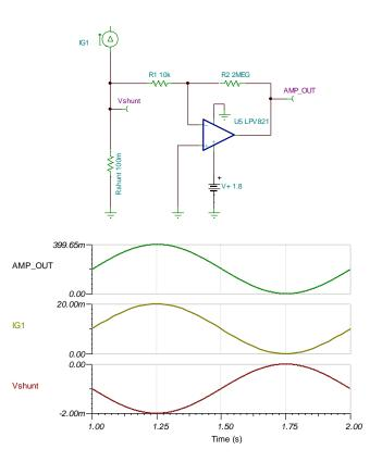
**Figure 3. Precision Current Monitoring Simulation**
