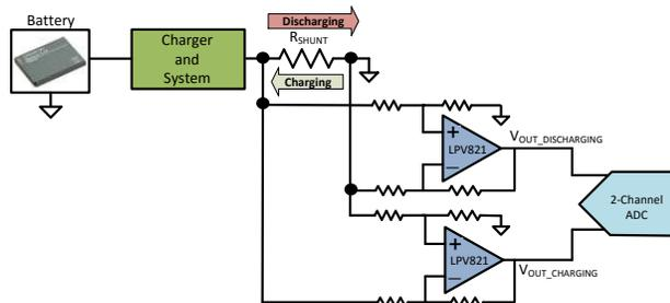
**Figure 4. Bidirectional Current Sensing**
