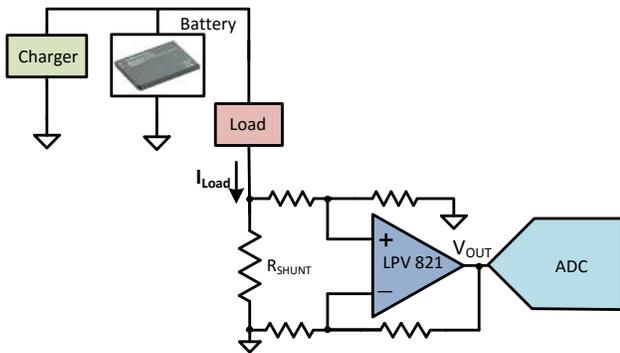
**Figure 3. Differential Amplifier Configuration**
