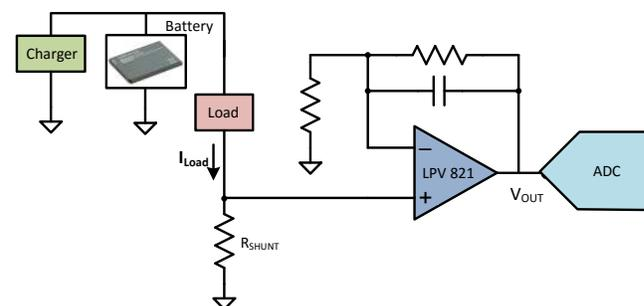
Figure 2. Single Ended Input Configuration
