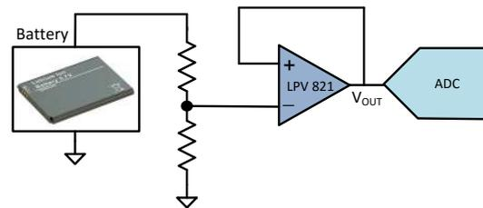
**Figure 5. Battery Voltage Monitoring**
