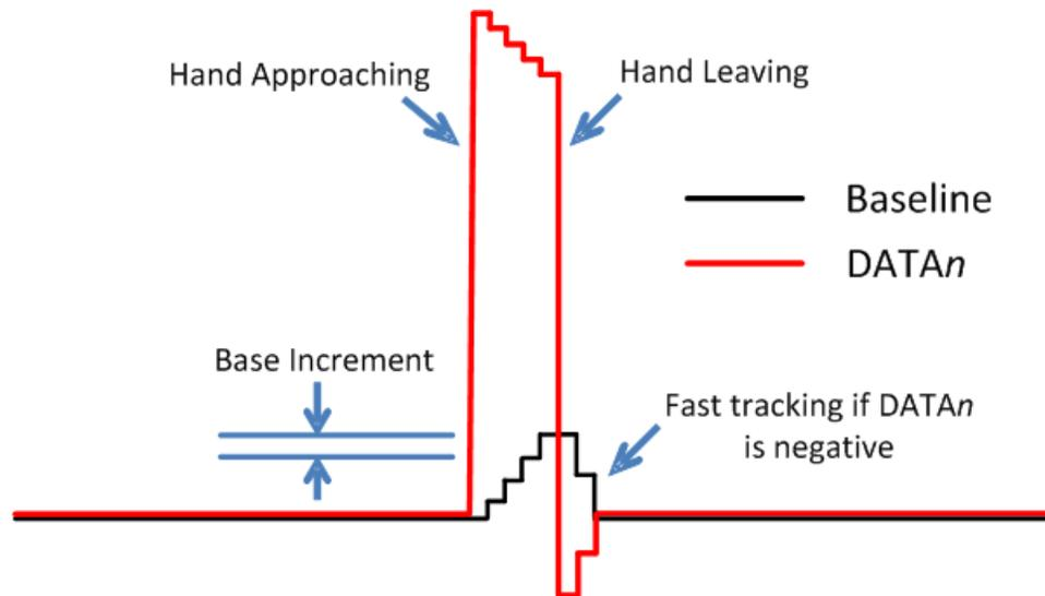
**Figure 3. Baseline Tracking for LDC2114 when a Hand Approaches the Sensor**
