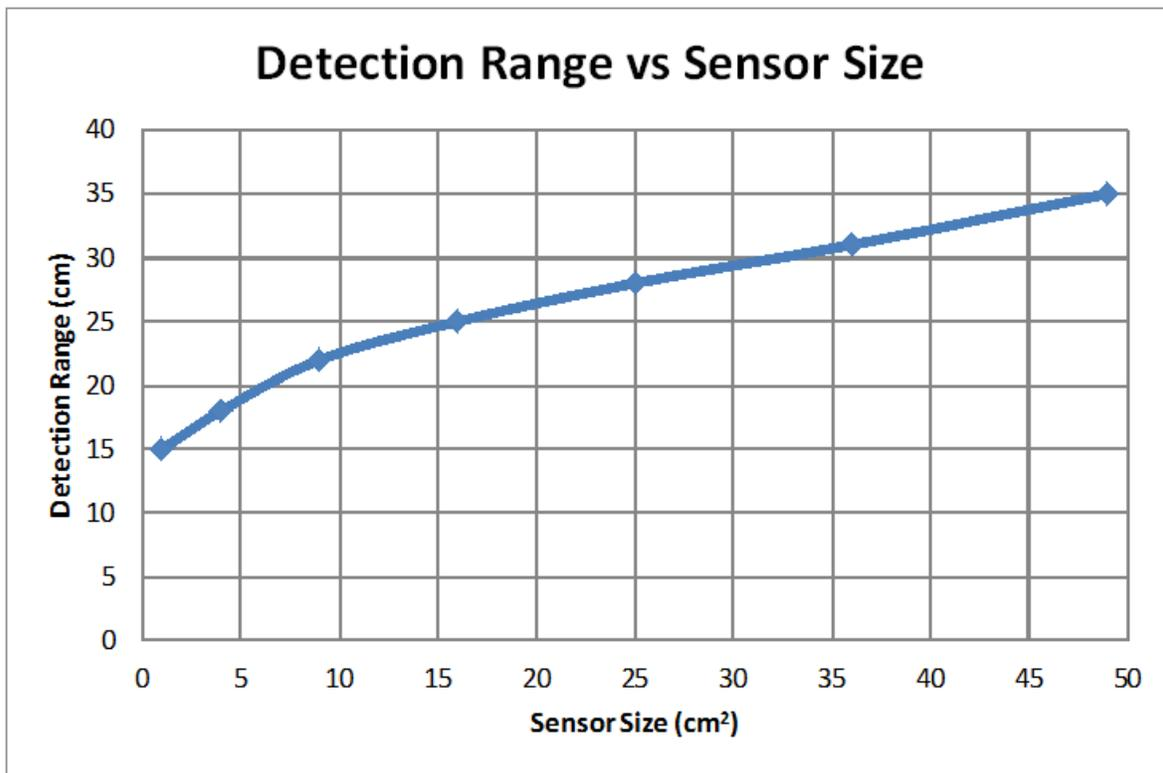
**Figure 4. Detection Range vs Square Sensor Size Using LDC2114**
