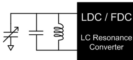
**Figure 1. Schematic of LC Resonance-Based Capacitive Sensing using LDC or FDC**
