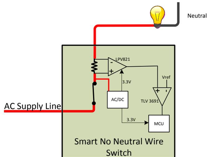
**Figure 6. Configuration With TLV3691 Comparator**
