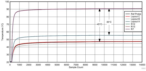
Figure 11. Layout A, B, C — 0.508-mm Distance
