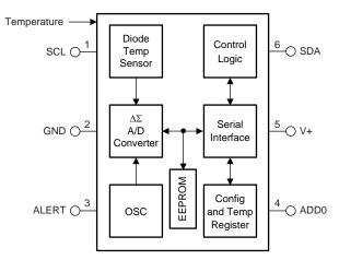
Figure 5. TMP116 Block Diagram
