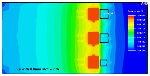
Figure 18. Layout D, E, F Thermal Air Gap 0.8-mm Slot Width
