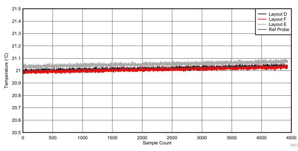
Figure 10. Layout D, E, F Ambient Air Temperature Measurement
