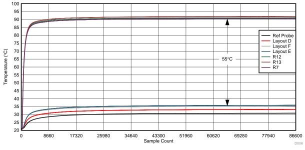
Figure 15. Layout D, E, F — 2.54-mm Isolation Air Gap
