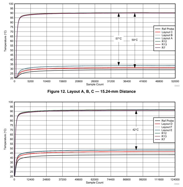
Figure 13. Layout D, E, F — 0.508-mm Distance
