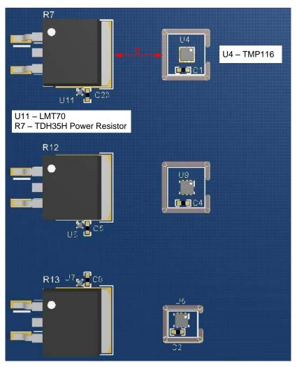
Figure 4. General Physical Layout for Test Board
