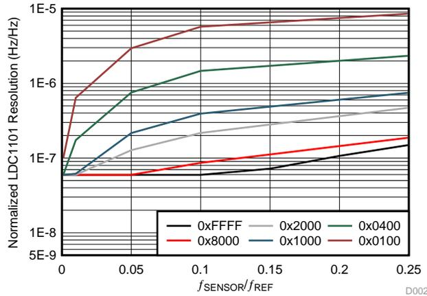
Figure 4. Normalized LDC1101 Resolution vs  $f_{\text{SENSOR}}$  and RCOUNT
