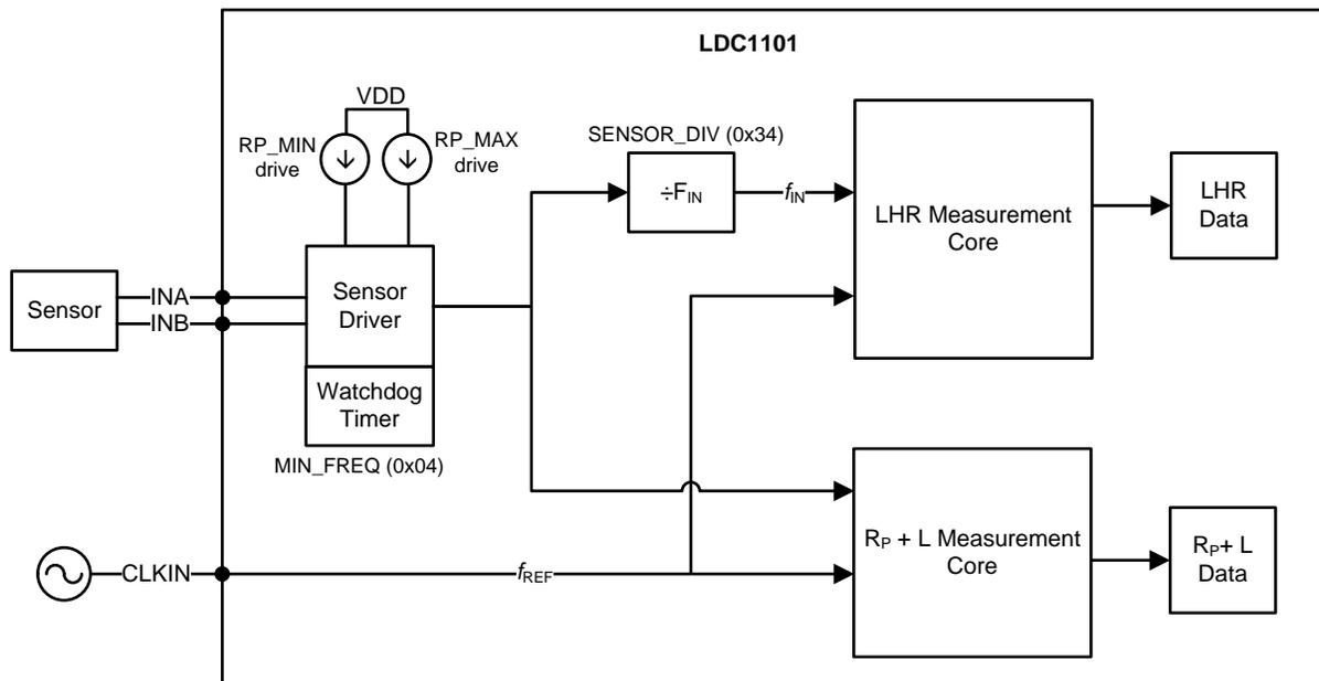
Figure 2. LDC1101 Clocking Diagram
