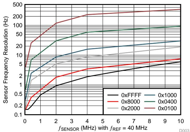
Figure 5. LDC161x Resolution with  $f_{\text{REF}} = 40 \text{ MHz}$
