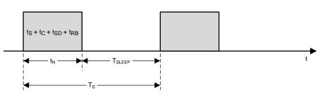
Figure 3. Duty Cycle as a Function of Settling Time, Conversion Time, Switching Time, and Readback Time
