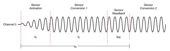
Figure 1. Single Channel Mode Sequencing in Continuous Conversion
