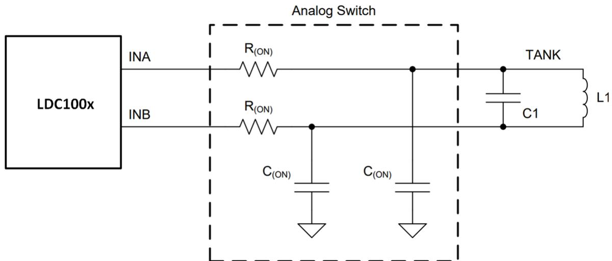
**Figure 3. Simplified Model of Analog Switch**
