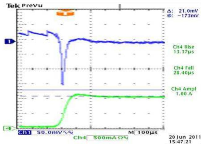
Figure 6. Expanded View of E-Load Transient Figure
