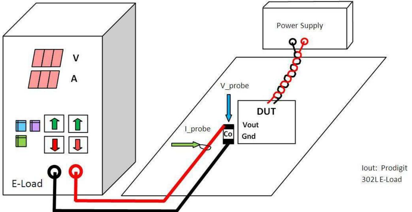
Figure 4. Using a Commercial Electronic Load Test Setup
