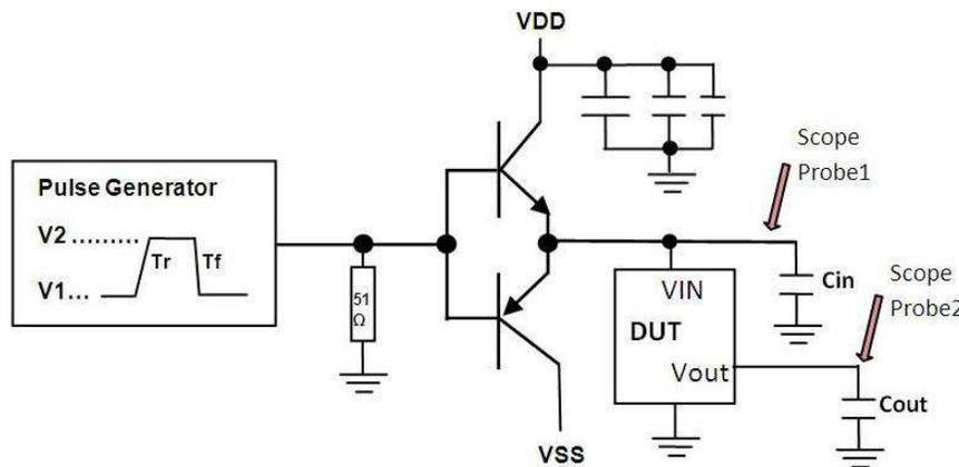
Emitter followers pair may use a single supply at VDD, allow sufficient margin to power the DUT VIN, and VSS is at ground potential. Adjust generator amplitude accordingly to accommodate the  $V_{be}$  drop or rise.
