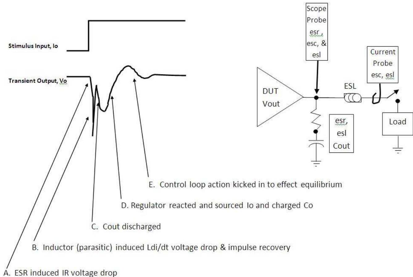
**Note:** Should not be concerned on the negative excursion if you have low parasitic L or fast stimulus edge rates  $v=L*di/dt$ . May observe a few mV if  $t_r > \text{few } \mu s$ , or few hundred mV if  $t_r < 200ns$  on a good layout/wiring platform.
