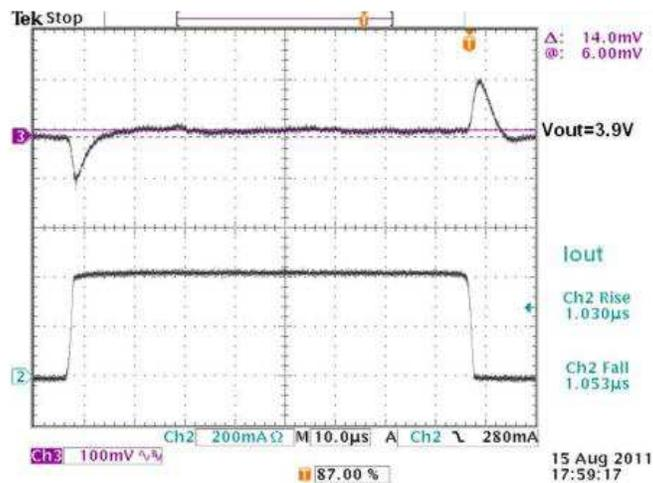
Figure 17. Integrated Load Transient Probe Jig @ Tr = 1µs
