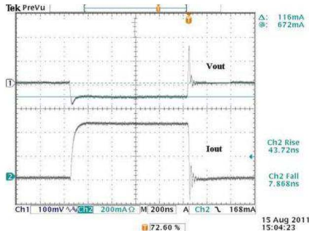
Figure 15. Integrated Load Transient Probe Jig @ Tr = 43.7 ns
