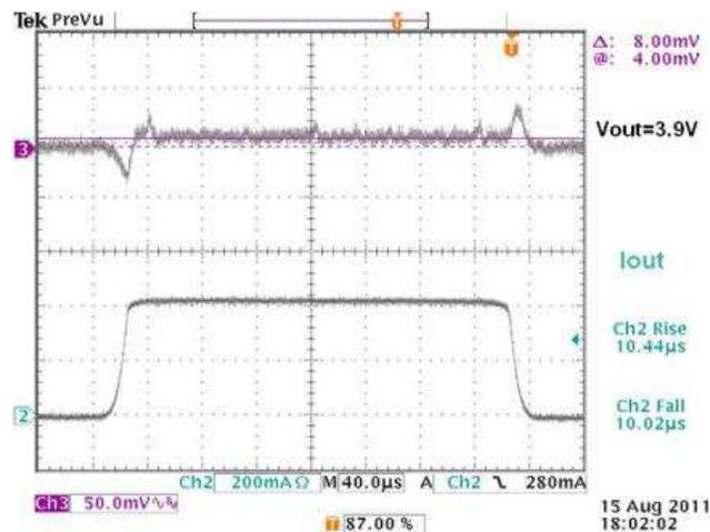
Figure 18. Integrated Load Transient Probe Jig @ Tr = 10 µs
