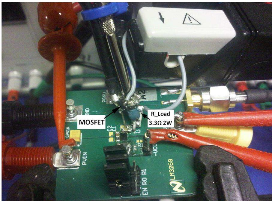
Figure 12. Load Transient Scope Probe Jig Assembly
