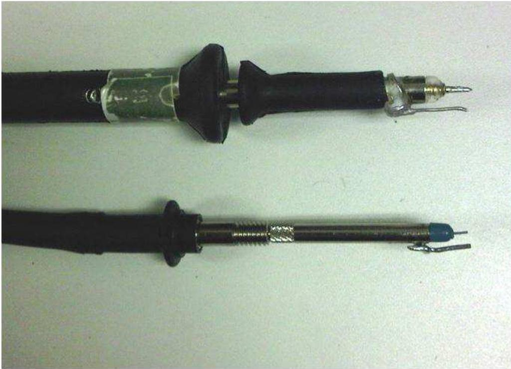
Figure 11. Scope Probes with Short Ground Tips
