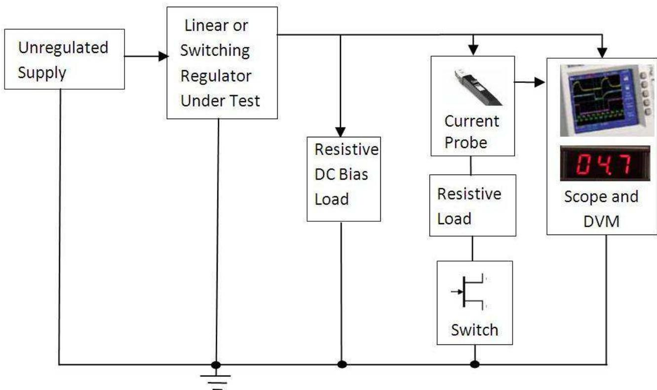
**Figure 1. Principle of a Load Transient Test Circuit**
