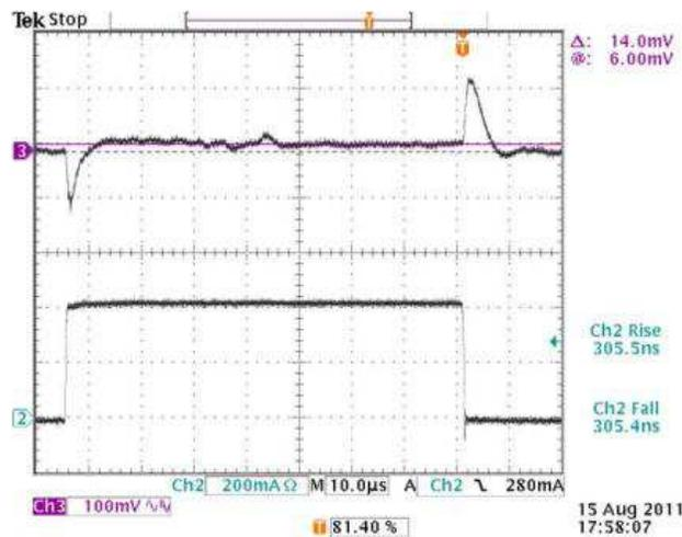
Figure 16. Integrated Load Transient Probe Jig @ Tr = 305 ns
