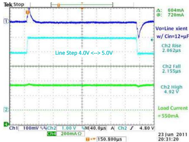
**Figure 23. Line Transient Jig 1.0V Step Driving a Buck w/C<sub>IN</sub>=12 µF**
