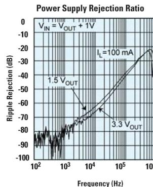
**Figure 4. LP5900 150 mA Low Dropout Linear Regulator PSRR Over Frequency**
