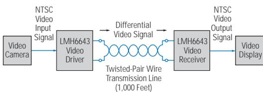
Figure 1: Block Diagram of Twisted-Pair Video System
