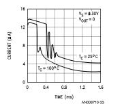
FIGURE 23. Output short-circuit current is reduced when power transistor junction temperature reaches 230°C and power limit takes over.
