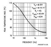
FIGURE 29. Peak junction-temperature rise as a function of frequency with an op amp driving a resistive load under conditions of worst-case dissipation.
