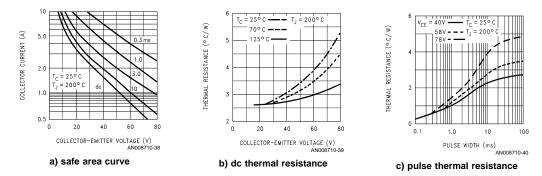
FIGURE 26. The worst-case power ratings of the output transistors are described by a) a safe area curve, b) the change in dc thermal resistance with temperature and operating voltage and c) the pulse thermal resistance.
