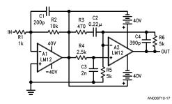
FIGURE 13. Cascading two op amps doubles output swing. Output may be increased by any number of stages, but a separate floating supply is required for each.
