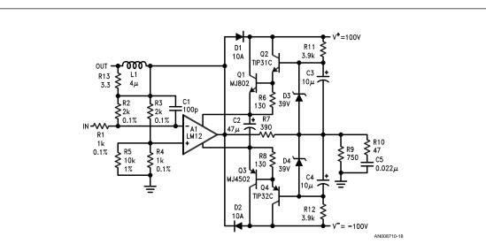
FIGURE 11. This amplifier can drive ±90V at ±10A, more than twice the output swing of the LM12. The IC provides current and power limiting for the discrete transistors.
