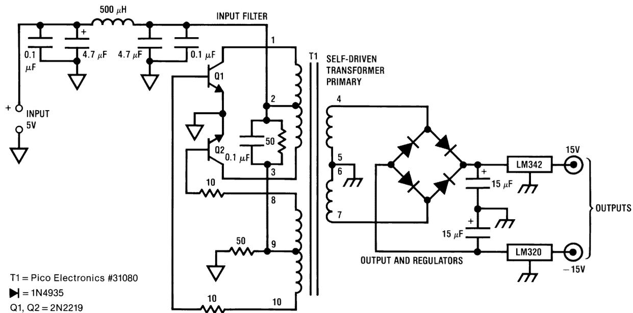
Figure 1. Typical DC-DC Converter
