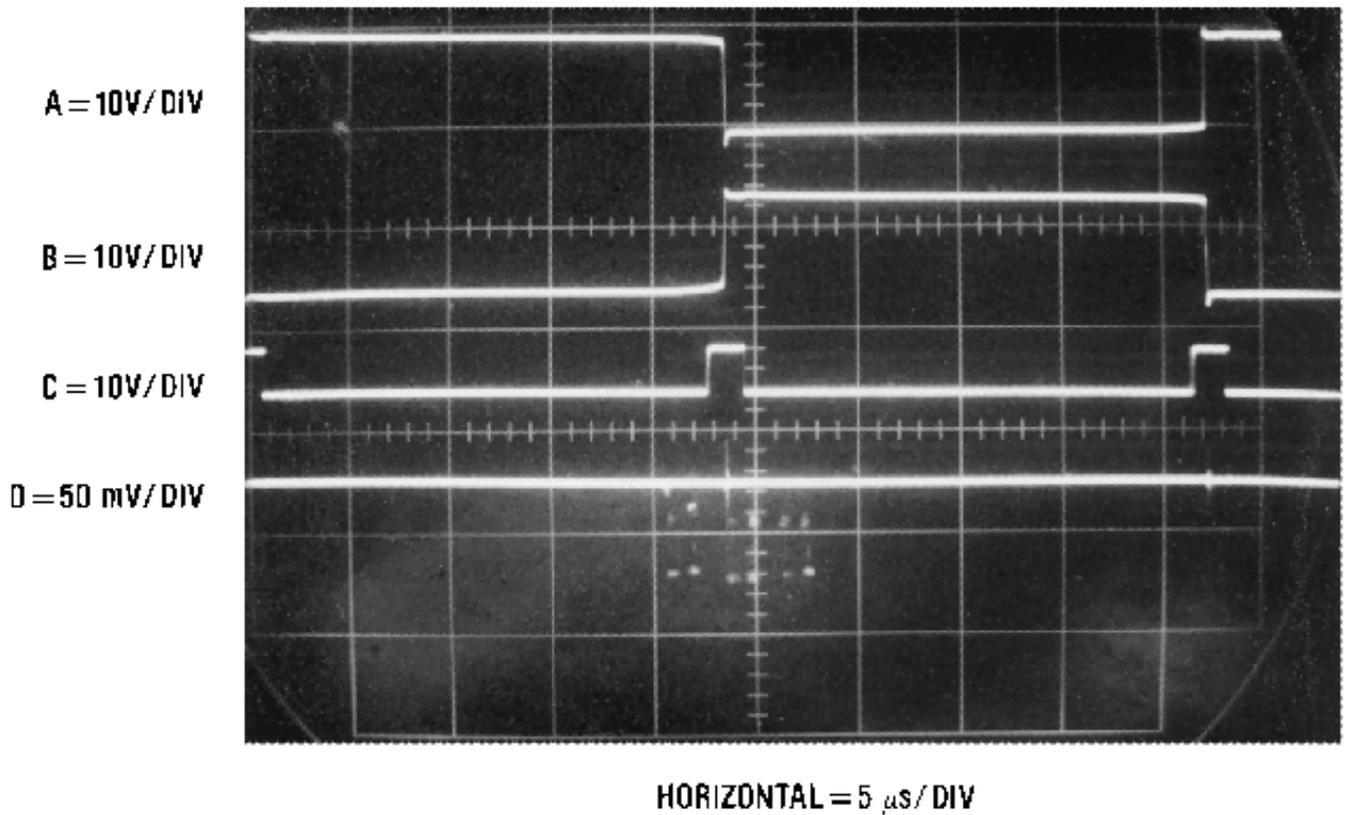
Figure 4. Switching Transistor Waveforms (A and B),Blank Pulse (C), and Converter Output Noise (D)
