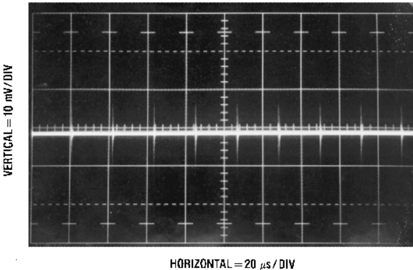
Figure 2. Typical Output Noise of Commercial DC-DC Converter
