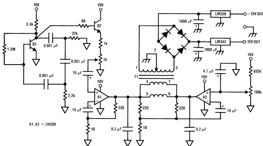
Figure 7. Sine Wave Driven Converter
