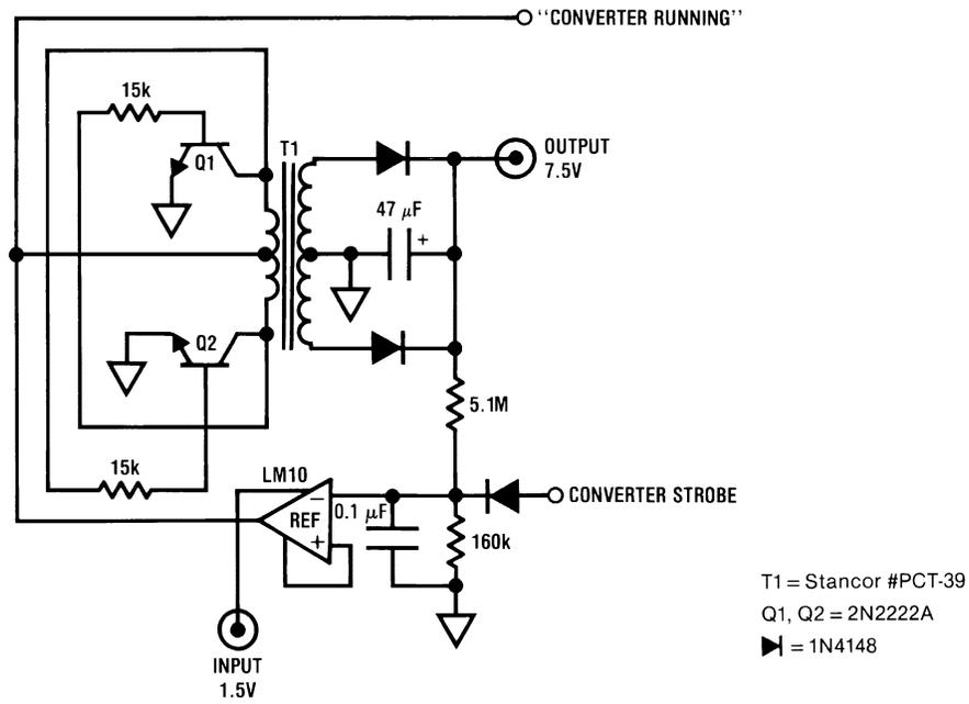
Figure 9. Low Power Converter
