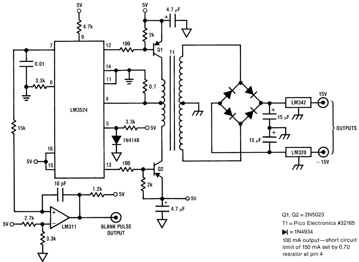
Figure 3. Blank Pulse Converter
