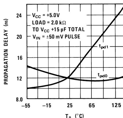
Figure 2. Delay vs Temperature
