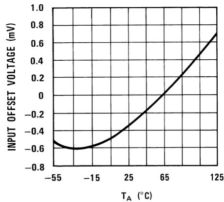
**Figure 3. Offset Temperature Coefficient**
