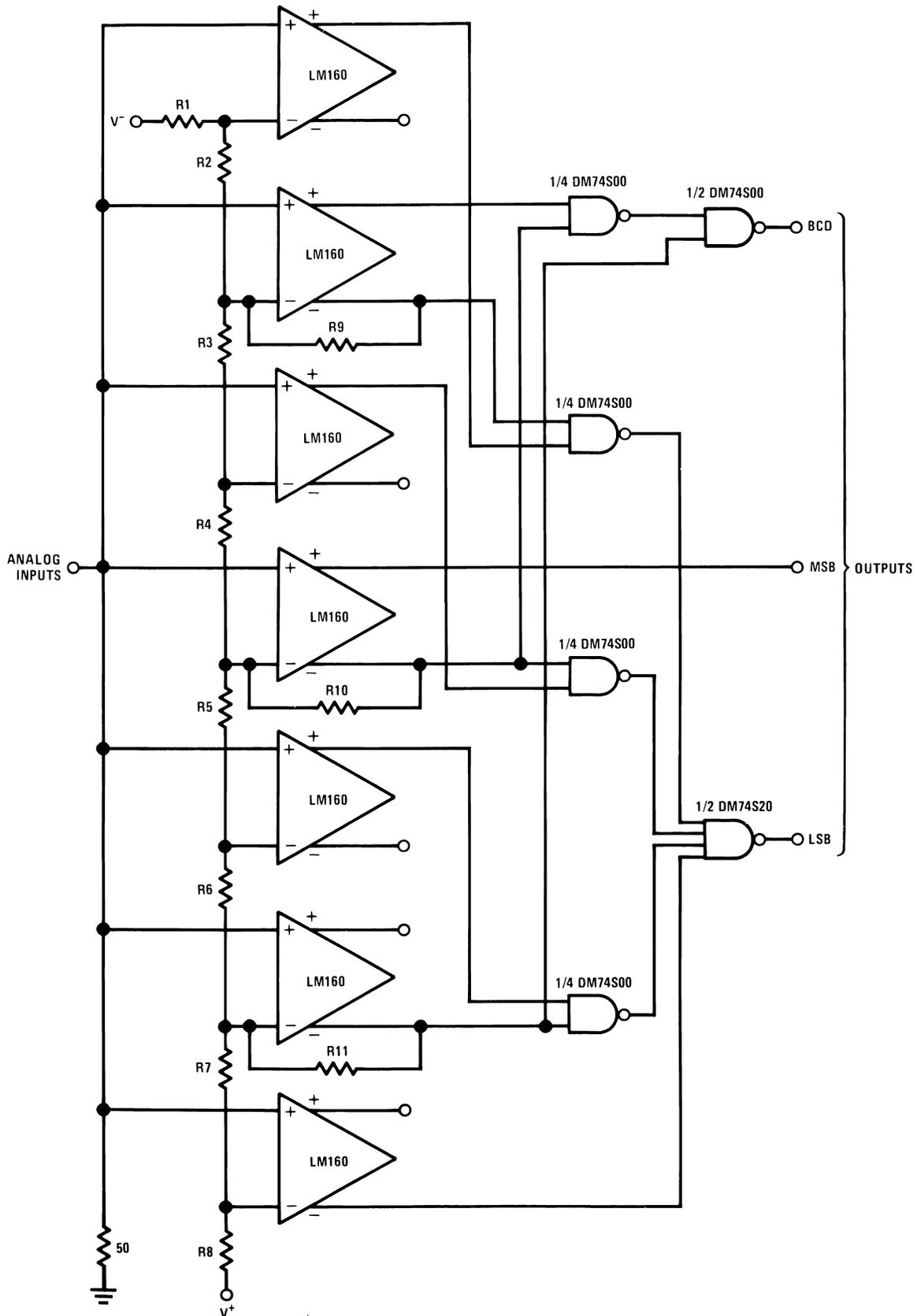
Figure 8. High Speed 3-bit A to D Converter
