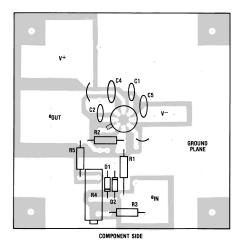
FIGURE 7. Single-Sided Sample PC Layout for LH0024
