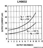
FIGURE 21. Continuous Output Drive Capability
