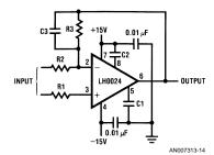
FIGURE 12. LH0024 Frequency Compensation Circuit
