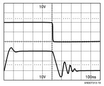
FIGURE 17. LH0032 Unity Gain Non-Inverting Large Signal Pulse Response:  $T_A = 25^{\circ}C,\, C_C = 10 \text{ pF},\, C_A = 100 \text{ pF}$
