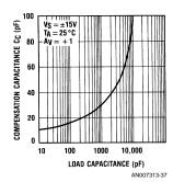
FIGURE 31. Frequency Compensation vs. Load Capacitance
