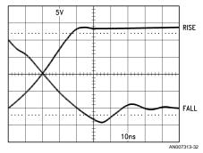
FIGURE 28. LH0032 Slew Response, Unity Gain Inverting Mode, Improved Compensation (C<sub>C</sub> = 5 pF, C<sub>A</sub> = 1000 pF)
