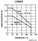
FIGURE 23. Maximum Power Dissipation
