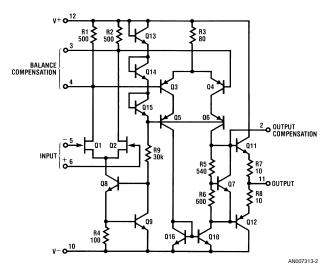
FIGURE 2. Complete LH0032 Schematic Diagram
