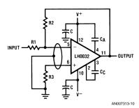
FIGURE 9. Guarding Inverting Figure Amplifier
