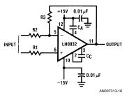
FIGURE 14. LH0032 Frequency Compensation Circuit
