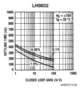
FIGURE 30. Settling Time vs. Closed-Loop Gain
