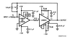
FIGURE 6. Wide Band Amplifier with 100 mA Output Capability
