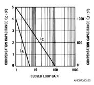
FIGURE 18. Recommended Value of Compensation Capacitor vs. Closed-Loop Gain for Optimum Slew Rate
