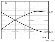
FIGURE 27. LH0032 Slew Response, Unity Gain Inverting Mode, Standard Compensation ( $C_C = 10$  pF,  $C_A = 100$  pF)
