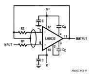
FIGURE 10. Guarding Non-Inverting Unity Gain Amplifier
