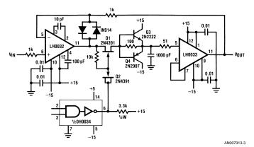
FIGURE 3. High Speed Sample and Hold Circuit
