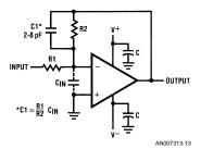
FIGURE 11. Compensating Amplifier Input Capacitance
