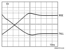
FIGURE 26. LH0024 Slew Response, Unity Gain Inverting Mode
