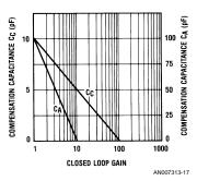
FIGURE 15. Recommended Value of Compensation Capacitor vs. Closed-Loop Gain for Optimum Settling Time
