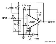
FIGURE 13. Input RC Lag Compensation Circuit
