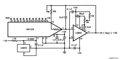
FIGURE 5. Fast Settling DAC
