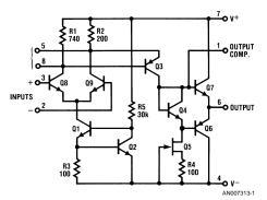
FIGURE 1. Complete LH0024 Schematic Diagram
