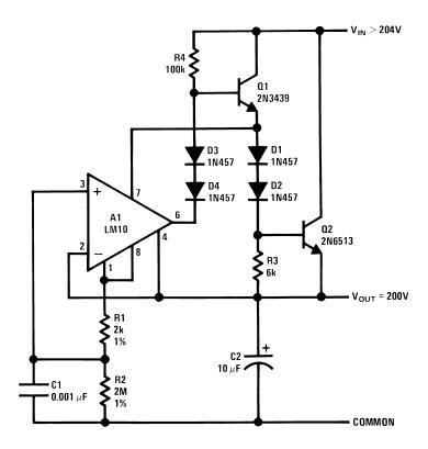
Figure 25. High-Voltage Regulator
