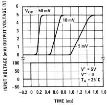
Figure 6. Comparator Response Times for Various Input Overdrives
