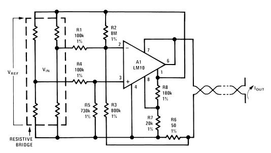
Figure 17. Two-Wire Transmitter for Resistive Bridge
