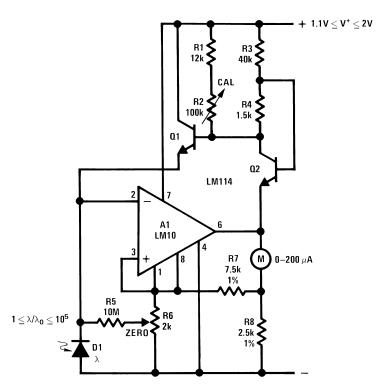
Figure 33. Logarithmic Light-Level Meter
