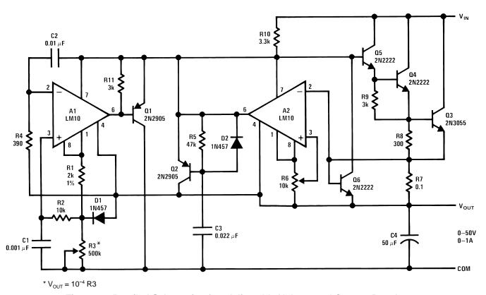
Figure 24. Detailed Schematic of an Adjustable Voltage and Current Regulator
