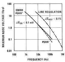
Figure 15. Noise Rejection for the Various Elements of Figure 16. Noise Frequency and Amplitude Required to Give Indicated Error
