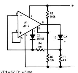
Figure 29. Battery Level Indicator with Regulated LED Current
