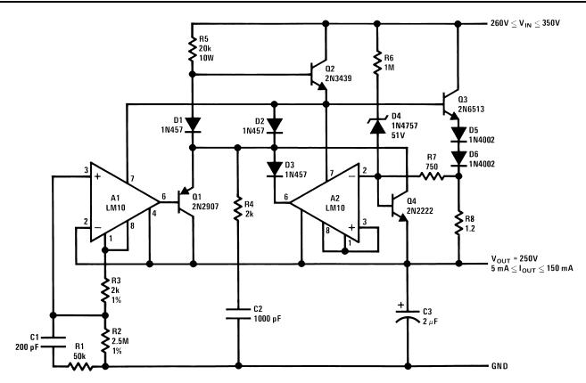
Figure 26. High Voltage Regulator with Foldback Current Limit
