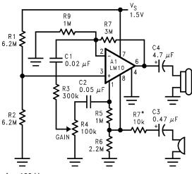
$Z_{OUT} \sim 680\Omega$ , @5 kHz,  $A_{V} \le 1$ k,  $f_{1} \sim 100$  Hz,  $f_{2} \sim 5$  kHz,  $R_{I} \sim 500$ . \* max gain trim
