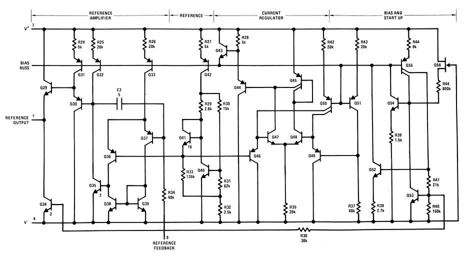
Figure 38. Simplified Schematic of the Reference and Internal Current Regulator
