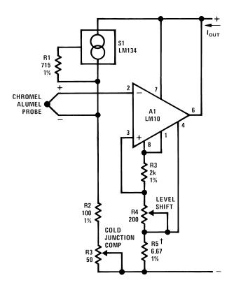
$200^{\circ}\text{C} \le \text{T}_{\text{p}} \le 700^{\circ}\text{C}$ 1 mA  $\le \text{I}_{\text{OUT}} \le 5$  mA † gain trim
