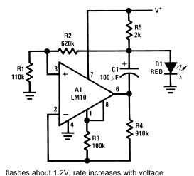
Figure 30. Undervoltage Indicator for Single Call
