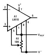
Figure 3. Op Amp Offset Adjustment
