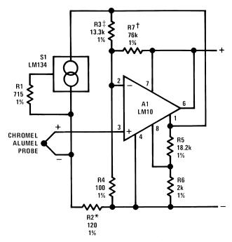
$4V \le V_{OUT} \le 20V$   $200^{\circ}C \le T_{p} \le 700^{\circ}C$ † span trim
