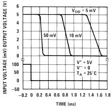
Figure 7. Comparator Response Times for Various Input Overdrives
