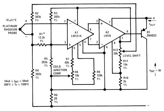
Figure 20. Precision Thermocouple Amplifier/Transmitter
