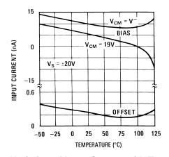
Figure 2. Variation of Input Current with Temperature
