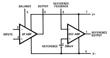
Figure 1. Functional Diagram of the New IC
