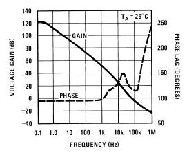
Figure 35. Open Loop Frequency Response
