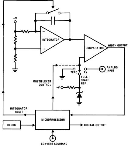
Figure 1. Dual-Slope Converter
