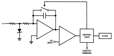
Figure 8. Single-Slope Integrating Converter
