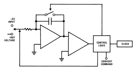
Figure 9. Dual-Slope Integrating Converter
