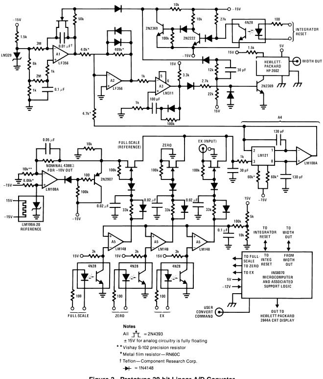
Figure 2. Prototype 20-bit Linear A/D Conveter
