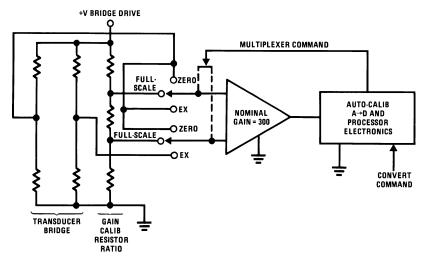
Figure 7. Block Diagram of the Converter Used to Generate a 15-bit Output Directly from a 30 mV Full-Scale Input
