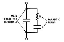
Figure 10. Modeling Parasitic Series RC Across the Terminals of the Main Capacitor
