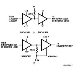
FIGURE 15. Input/Output Level Shifters
