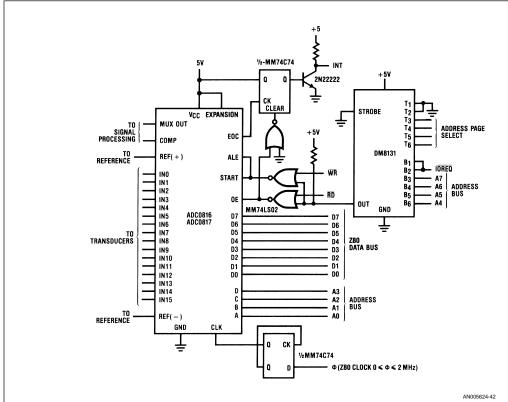
NOTE: PULL-UP RESISTORS SHOULD BE ADDED TO CMOS INPUTS TO IMPROVE TTL COMPATABILITY
