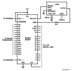
FIGURE 20. Sample/Hold Converter Using LF398
