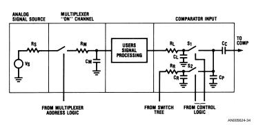
FIGURE 16. Simplified Multiplexer/Comparator Equivalent Circuit
