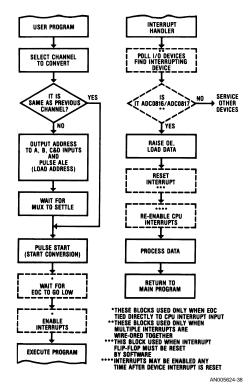
FIGURE 21. Flow Chart for Interrupt Control of ADC0816/ADC0817
