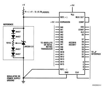
FIGURE 5. Simple Absolute Converter Using LM336-5.0 Converter
