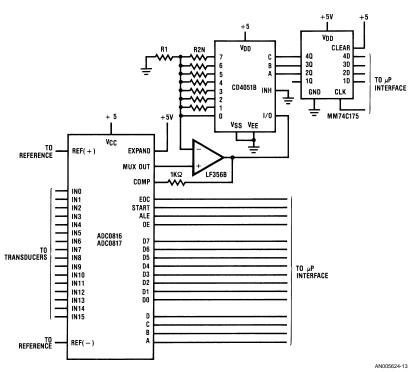
FIGURE 18. Microprocessor Controlled Gain
