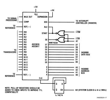
FIGURE 23. Simple INS8080/8224/8228 to ADC0816/ADC0817 Interface
