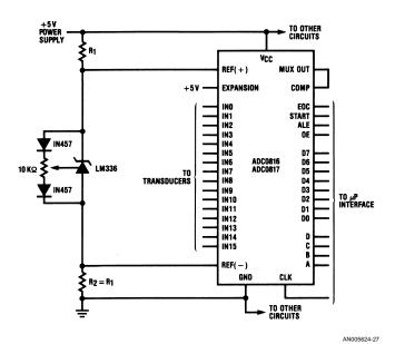
FIGURE 8. Supply Centered Reference Using LM336 2.5V Reference
