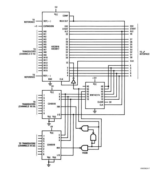
FIGURE 10. Simple 32-Channel A/D Converter
