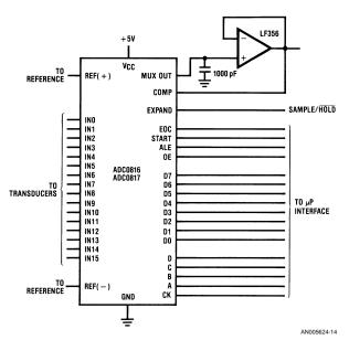
FIGURE 19. Op Amp Sample Hold Circuit
