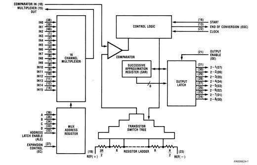
FIGURE 1. ADC0816/ADC0817 Functional Block Diagram
