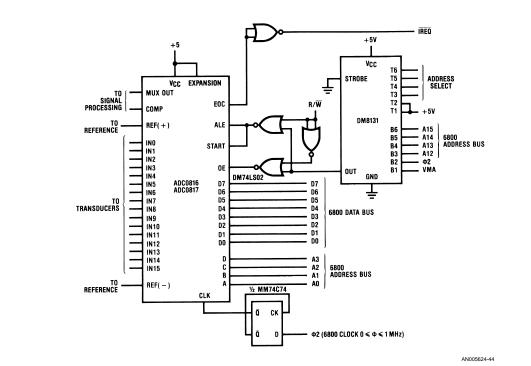
NOTE: PULL-UP RESISTORS SHOULD BE ADDED TO CMOS INPUTS TO IMPROVE TTL COMPATABILITY FIGURE 29. 6800 to ADC0816/ADC0817 Interface
