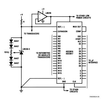
FIGURE 7. Buffered Reference Used as Power Supply
