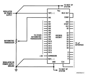
FIGURE 4. Simple Ratiometric Converter Using Power Supply as Reference
