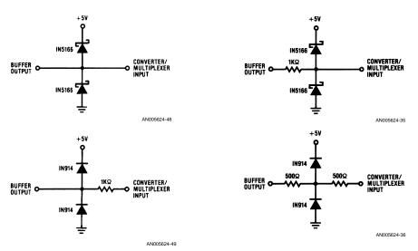
FIGURE 17. Analog Input Protection Circuitry
