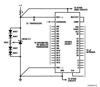
FIGURE 6. Reference Used as Power Supply
