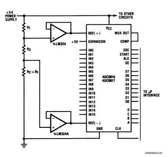
FIGURE 9. Supply Centered Reference Using Buffered Resistor Divider
