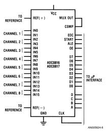
FIGURE 11. Simple 8-Differential Channel Converter
