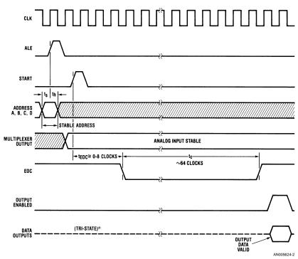
FIGURE 3. ADC0816/ADC0817 Timing Diagram
