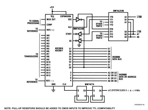
NOTE: PULL-UP RESISTORS SHOULD BE ADDED TO CMOS INPUTS TO IMPROVE TTL COMPATABILITY
