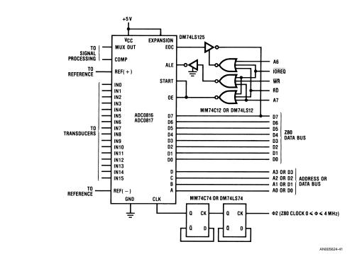
NOTE: PULL-UP RESISTORS SHOULD BE ADDED TO CMOS INPUTS TO IMPROVE TTL COMPATABILITY FIGURE 25. Simple Z80 Interface to ADC0816/ADC0817
