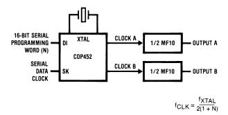
Figure 3. Programmable Dual Clock Generator
