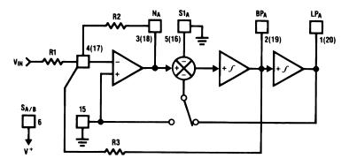
Figure 5. MODE 1: Notch, Bandpass, and Lowpass
