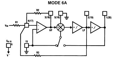
Figure 11. MODE 6A: Single Pole, Highpass, and Lowpass
