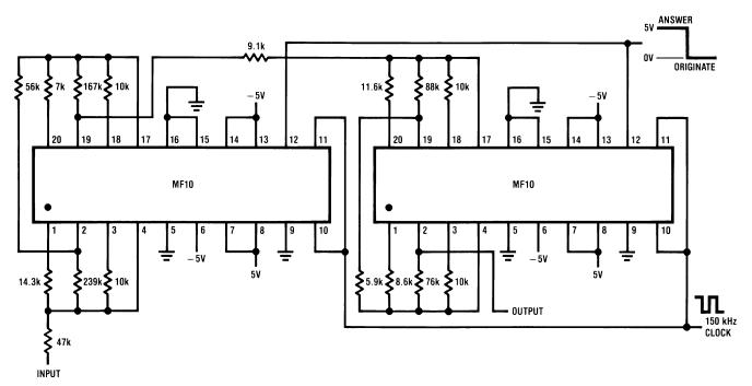
Figure 16. Complete Full-Duplex 300 Baud Modem Filter
