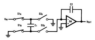
Figure 19. Non-Inverting Integrator Used in the MF10
