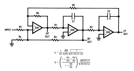
Figure 1. Universal State Variable 2nd Order Active Filter (note the complexity of design equations and the number of critical external components)
