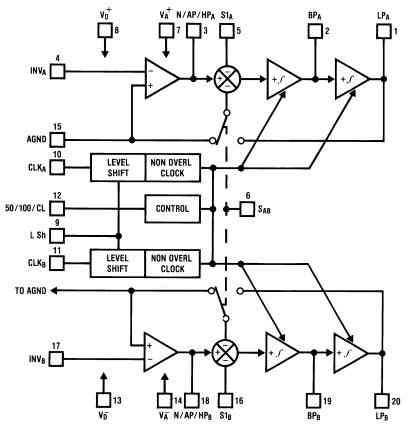
Figure 2. Block Diagram of the MF10
