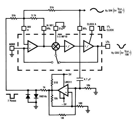
Figure 15. Generating Quadrature Sine Waves from a T<sup>2</sup>L Clock
