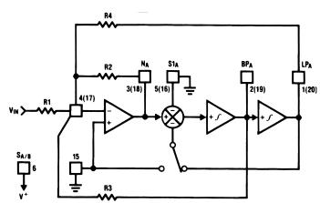
Figure 6. MODE 2: Notch (with  $f_n \le f_o$ ), Bandpass, and Lowpass
