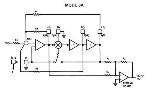
Figure 8. MODE 3A: Highpass, Bandpass, Lowpass, and Notch
