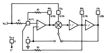
Figure 9. MODE 4: Allpass, Bandpass, and Lowpass
