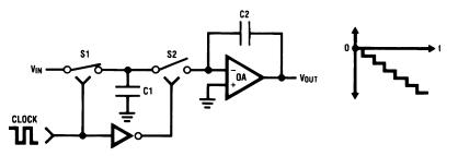
Figure 18. Inverting Integrator with Input Resistor Replaced with 2 Switches and Capacitor
