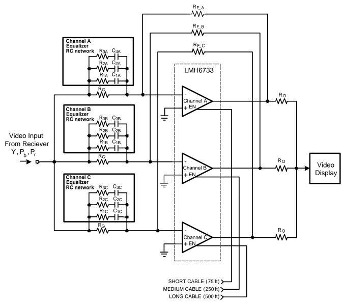
Figure 6. Equalization Circuitry for Various CAT5 Cable Lengths
