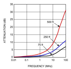
Figure 1. CAT5 Cable Attenuation
