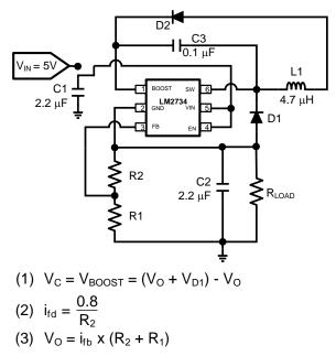
Figure 9. LMH2734 Circuit and Equations for -5 V Supply Generation
