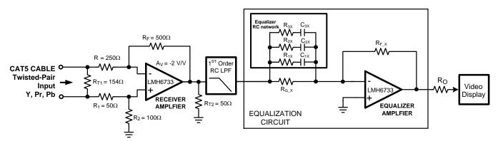
Figure 5. CAT5 Video Receiver and Equalization Circuit
