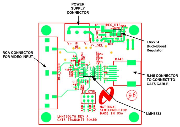
Figure 4. CAT5 Transmit Board
