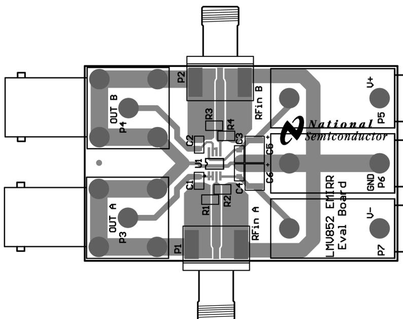
Figure 5. Layout for LMV852, All Layers
