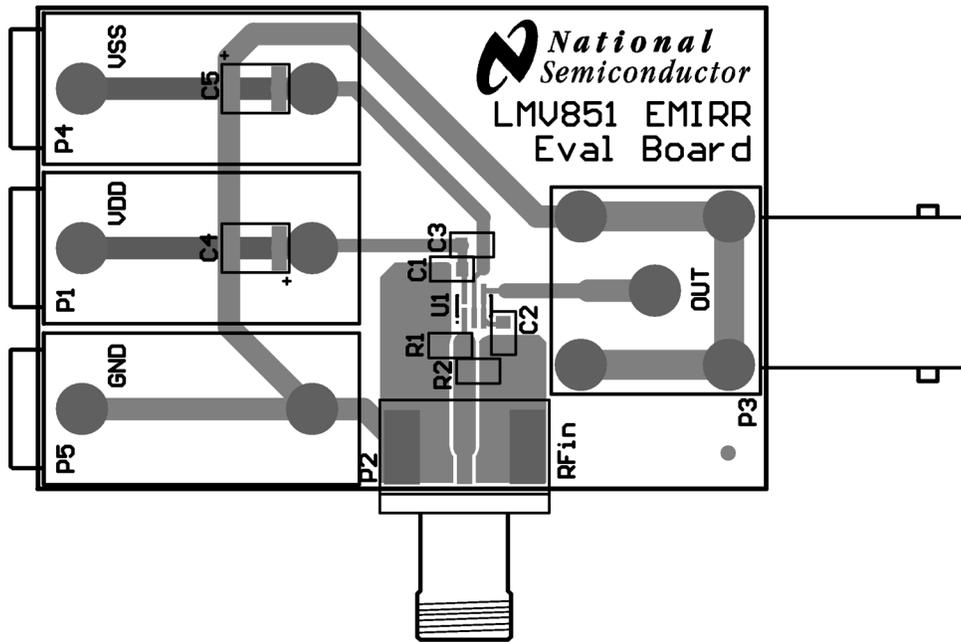
Figure 2. Layout for LMV851, All Layers
