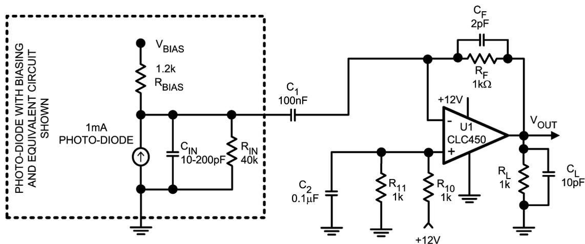
**Figure 1. Single-Supply Photo-Diode Amplifier Using CLC450 Current-Feedback Amplifier**
