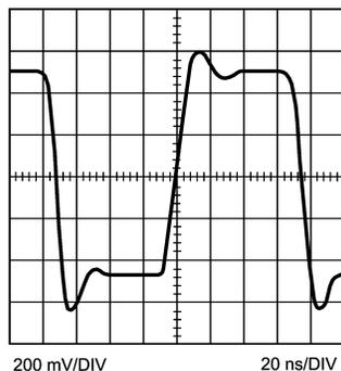
Figure 4. Output Step Response 20 ns/div, 0.2 V/div
