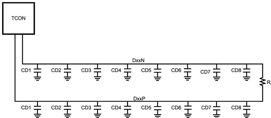
**Figure 11. Loading of RSDS Bus**
