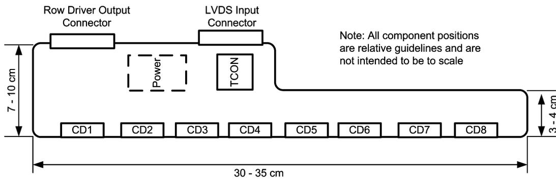
Figure 13. Typical PCB Size and Functional Grouping
