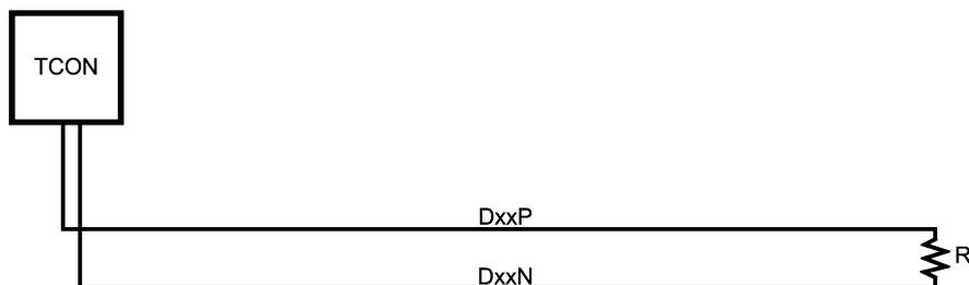
Figure 4. L-Configuration Termination Scheme
