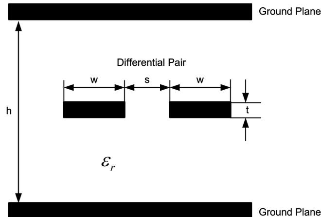
**Figure 8. Dimensions for Calculating Stripline Impedance**
