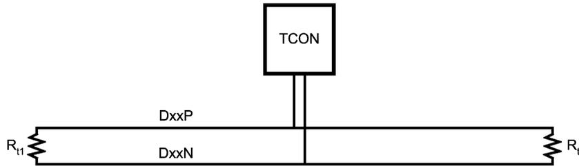
Figure 2. T-Configuration Termination Scheme
