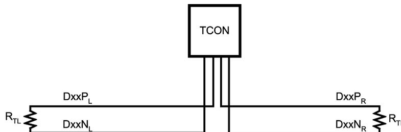
Figure 6. Dual Bus Configuration Termination Scheme
