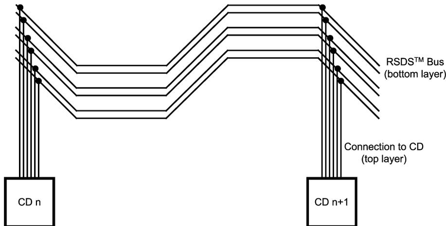
Figure 10. Enlarged View of RSDS Bus Routing
