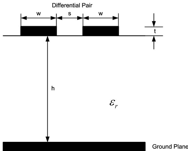
Figure 7. Dimensions for Calculating Microstrip Impedance
