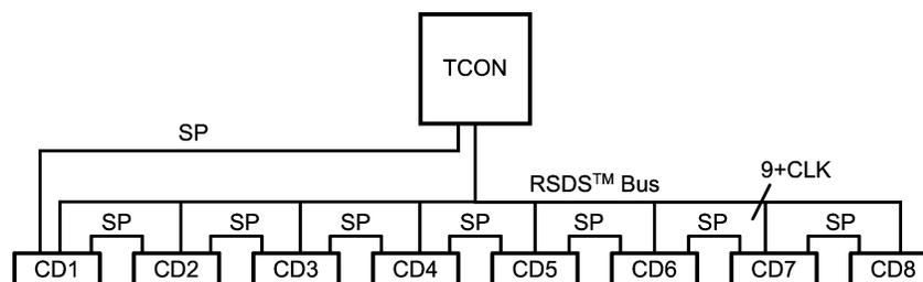
Figure 1. T-Configuration (XGA System)
