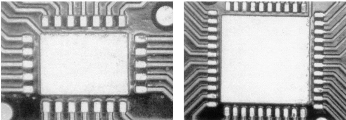
**Figure 26. Pads After Removing Components and Cleaning**
