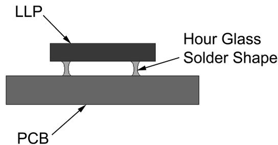
**Figure 25. Pullback LLP Hour Glass Solder Joint**
