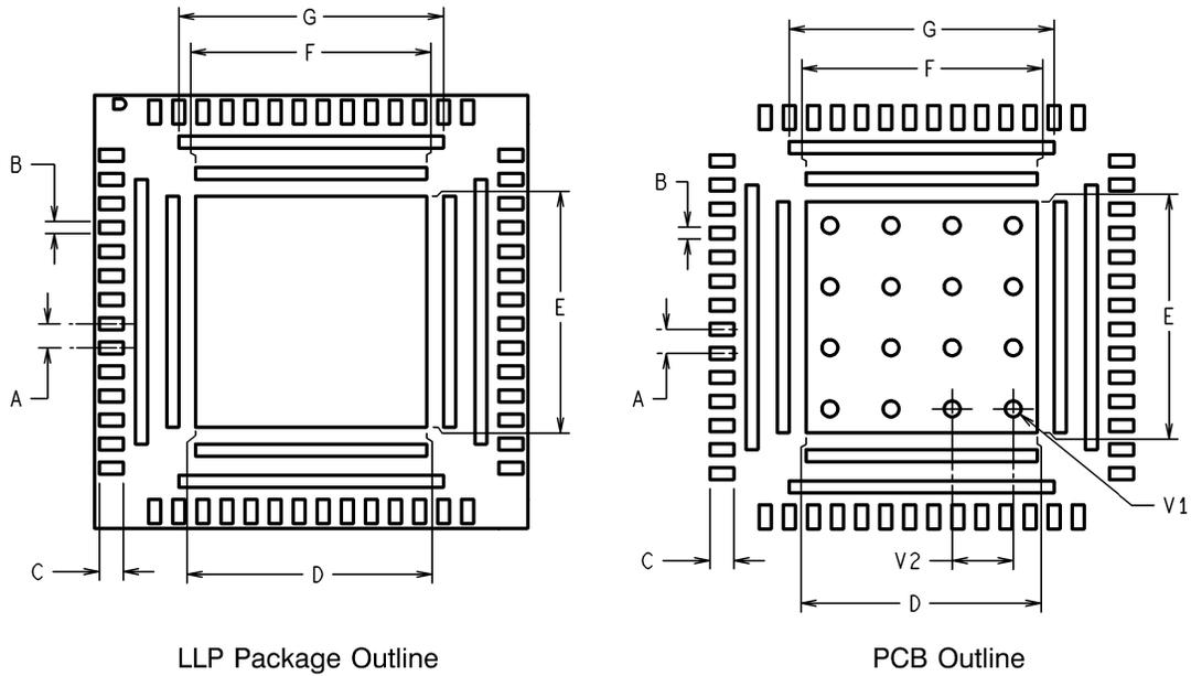
Dimensions A, B, C, D, E, F and G of PCB are 1:1 ratio with package pad dimensions. For specific detailed package dimensions refer to respective marketing outlines.
