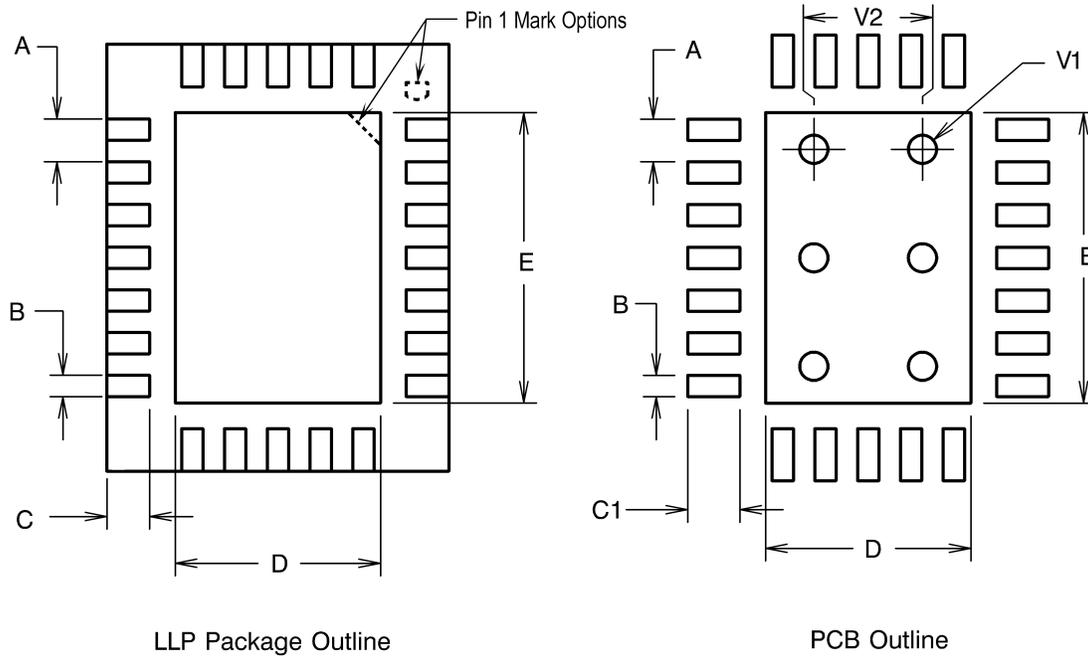
Dimensions A, B, D, and E of PCB are 1:1 ratio with package pad dimensions. For specific detailed package dimensions refer to respective marketing outlines.
