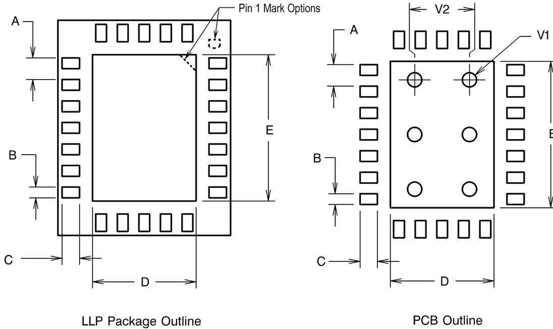
Dimensions A, B, C, D, and E of PCB are 1:1 ratio with package pad dimensions. For specific detailed package dimensions refer to respective marketing outlines.
