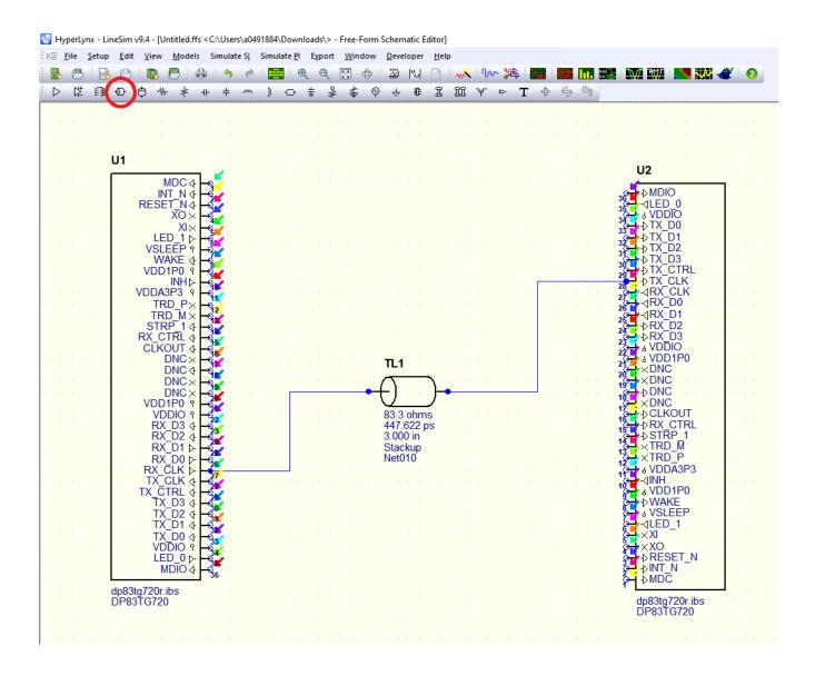
6. Double click TL1 and change the type to Simple. Set the transmission line parameters as desired. Click "OK."
