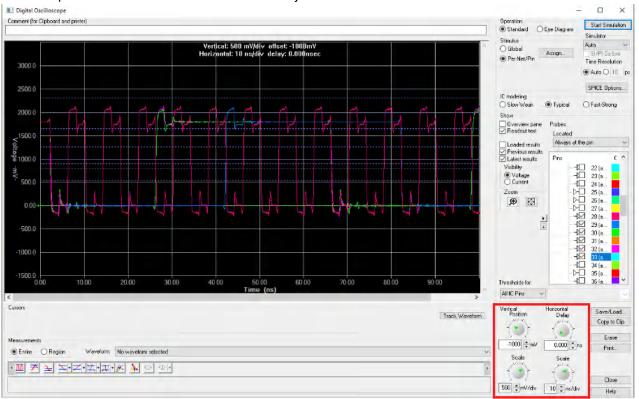
5. Any time or voltage value can be gathered from this plot manually. Click the Track Waveform button and click on a waveform. The cursor information will be shown here.
