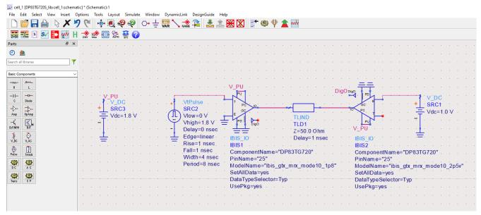
6. Now that the necessary connections are made, double click on the left IBIS component, and navigate to the Pin tab. Here, select the pin and available models. Select the RX\_CLK pin and use the default Model. Click Apply.
