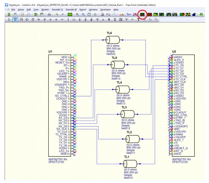
2. Select which pins to view waveforms of. Click the triangle to the left of the pins box and click "Disable all probes." Select pins 28-33 on U2.
