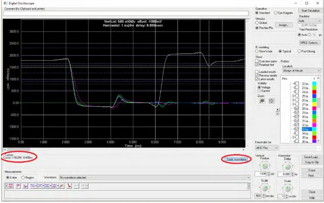
6. To acquire automatic measurements, select a waveform and measurement option in the bottom left. Options include peak-to-peak voltage, rise/fall times, positive/negative overshoot, etc.
