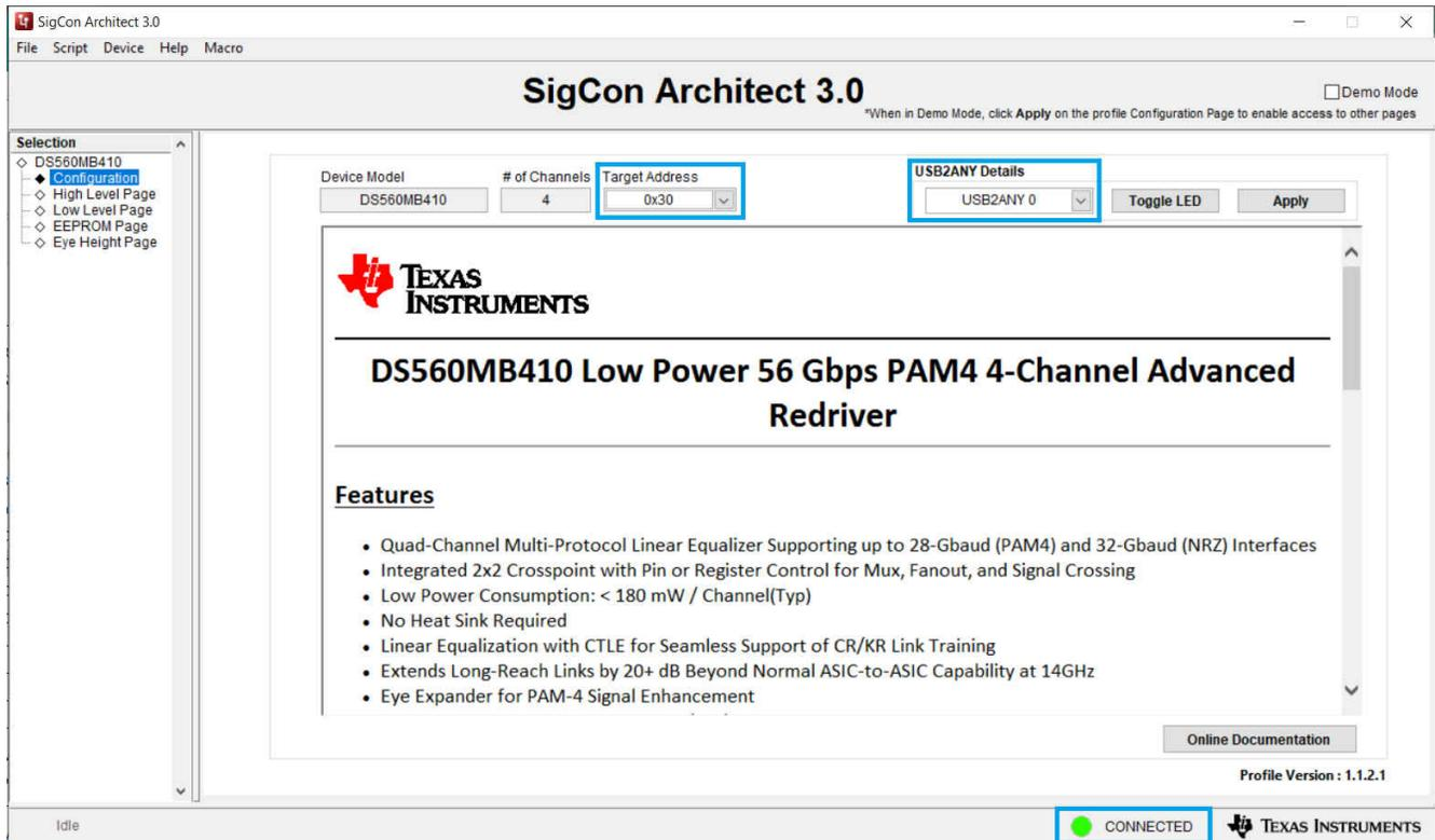
**Figure 5-5. Establishing a Connection with the DS560MB410**
