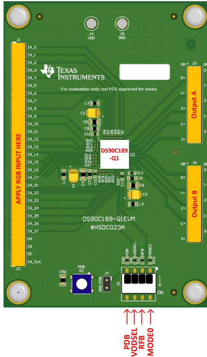
Figure 2. Demo Board Connections
