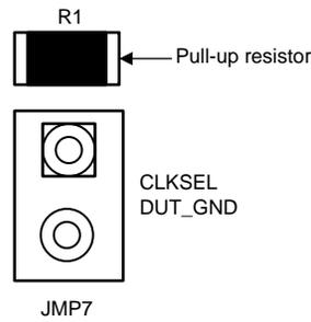
**Figure 2. Clock Rising Edge (High) Jumper Setting**
