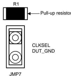
**Figure 3. Clock Falling Edge (Low) Jumper Setting**
