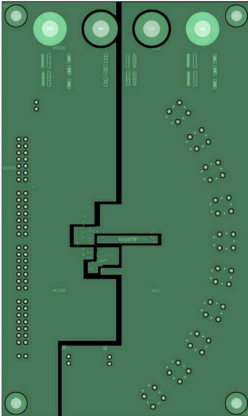
Figure 13. LVDS83BTSSOPEVM Layer 4 – V<sub>CC</sub>
