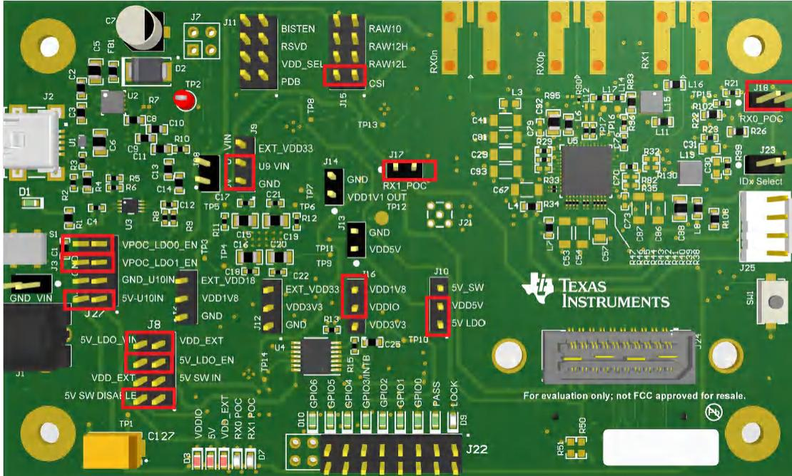
**Figure 3-32. DS90UB954-Q1EVM (or variant) With Highlighted Jumpers**
