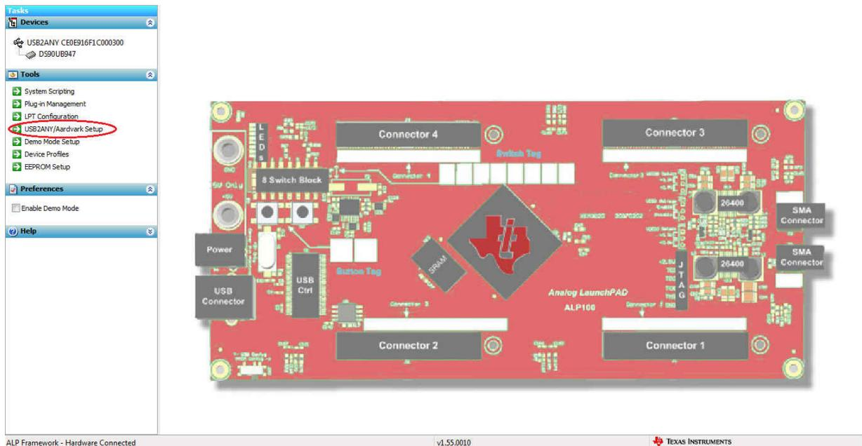
Figure 3-16. USB2ANY Setup
