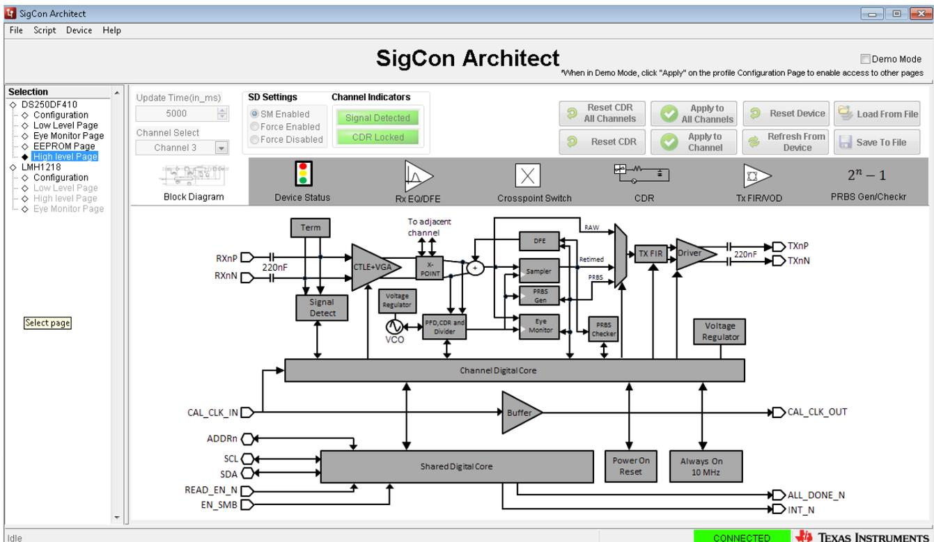
Figure 9. High-Level Page, with Block Diagram Tab Selected
