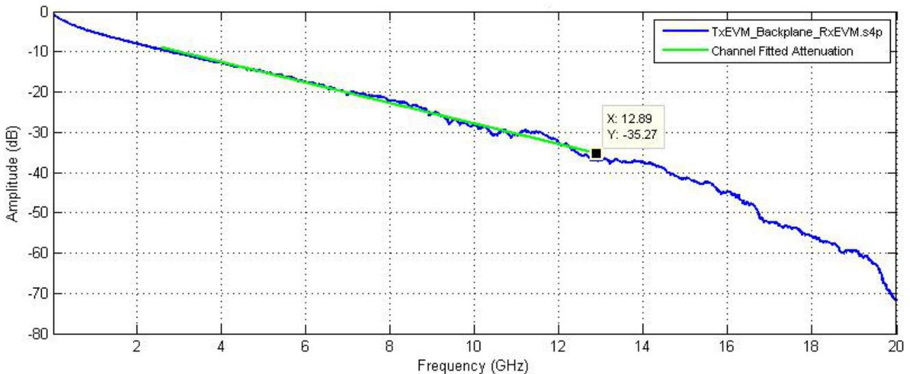
Figure 20. SDD21 Loss Characteristic of Example Test Case
