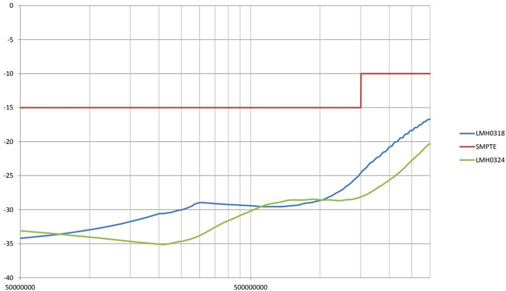
Figure 7. LMH0318 and LMH0324 Return Loss vs SMPTE Specification
